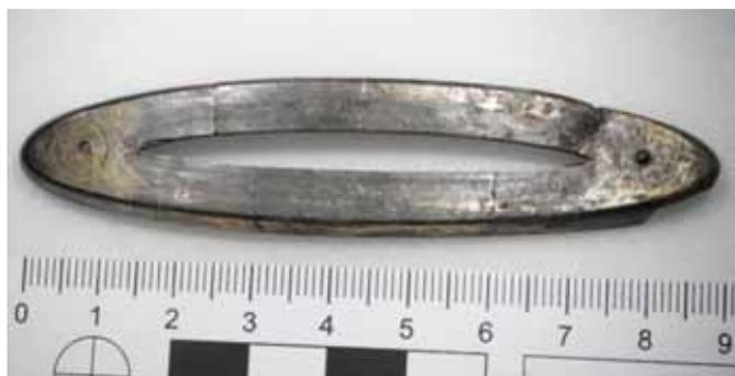
Surface XRF analysis was undertaken on the front of the hilt-plate in areas of gilding and areas with no observable gilding present, as well as the inside. Sub-surface analysis was carried out on the inside of both fragments.
