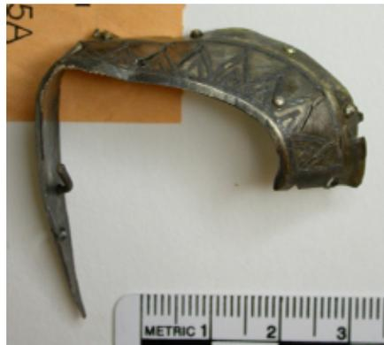
Surface XRF analysis was undertaken on the front of the niello mount and also on four pins. Sub-surface analysis was carried out on the back.
