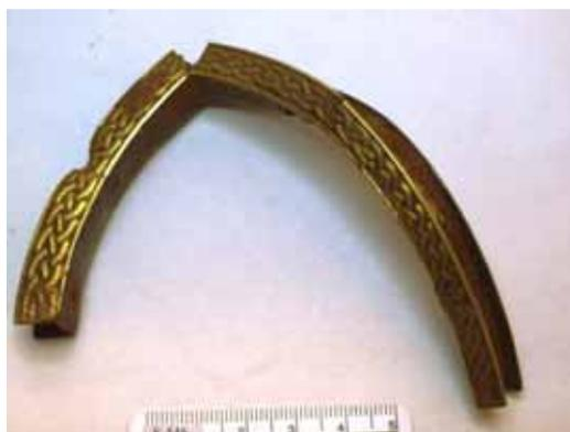
Surface XRF analysis was undertaken on the gilded front of the crest. Sub-surface analysis was carried out on the back.
