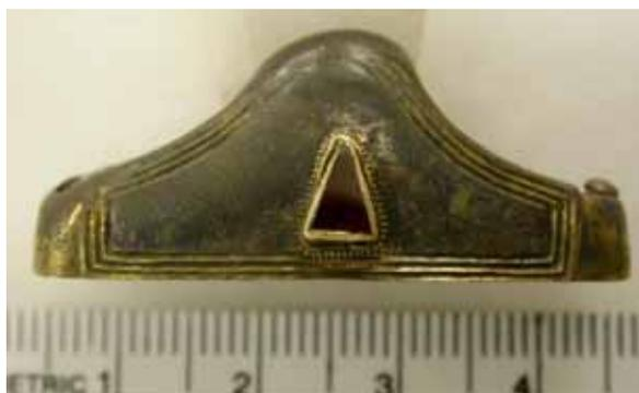
Surface XRF analysis was undertaken on the front gilding, the border around the garnet and the beaded wire on the pommel. Sub-surface analysis was carried out on the base.
