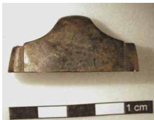
Surface XRF analysis was undertaken on the front of the pommel. Sub-surface analysis was carried out on the base.
