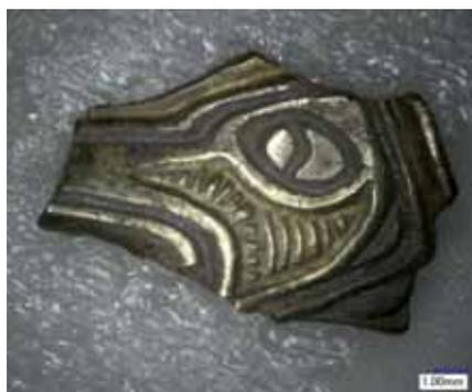
Surface XRF analysis was undertaken on the gilded front of the fragment. Sub-surface analysis was carried out on the inside.
