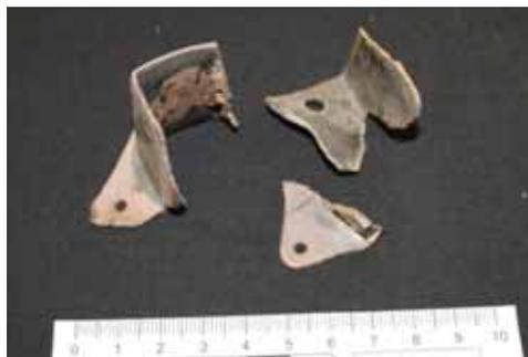
Surface XRF analysis was undertaken on the front of the bracket. Sub-surface analysis was carried out on the base.
