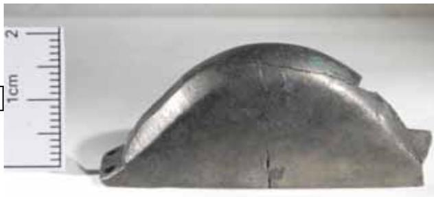
Surface XRF analysis was undertaken on the front of the pommel. Sub-surface analysis was carried out on the base.
