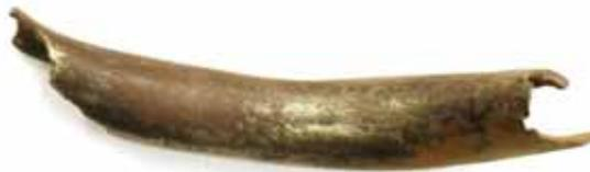
Surface XRF analysis was undertaken on the front of the c-tubing. Sub-surface analysis was carried out on the back.
