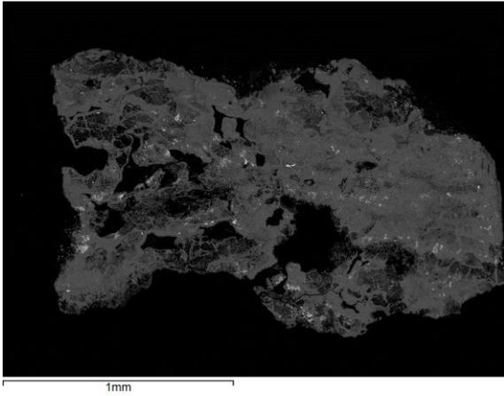
*Figure 15. SEM image of a cross-section sample from K355 showing the very porous nature of the material.*
