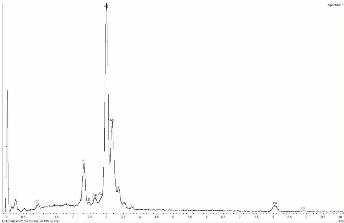
Figure 20. Typical SEM-EDS spectrum of the silver sulphide inclusions within the copper carbonate grains in sample from K355.
