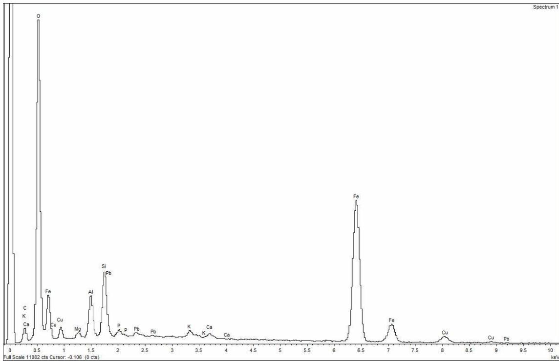
Figure 25. Typical SEM-EDS spectrum for the red area identified within the sample from K572, obtained on an unprepared surface.
