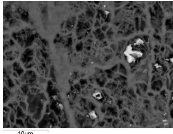
*Figure 18. Detail of the silver sulphides filling the pores of the copper-rich matrix in K355, under the SEM. See Figure 20 for a relevant EDS spectrum.*
