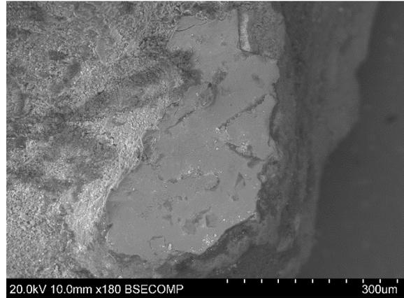
Figure 23. Detail of the red particle shown in Figure 22, as seen under the SEM. For an EDS spectrum of this area, see Figure 25.
