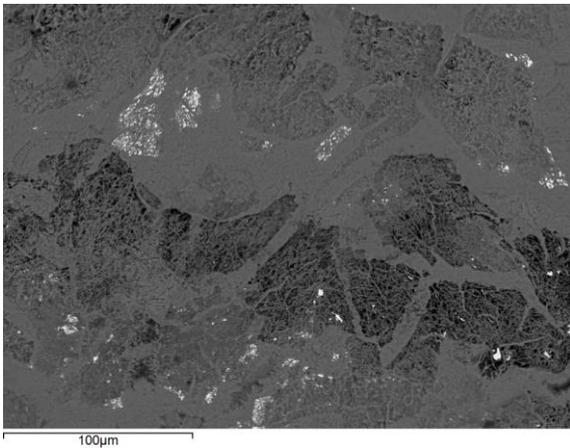
*Figure 17. SEM image of a cross-section sample from K355 showing the porous crystals of copper carbonate, with some cavities filled with bright silver sulphides. See Figure 19 for an EDS spectrum of the dominant phase.*
