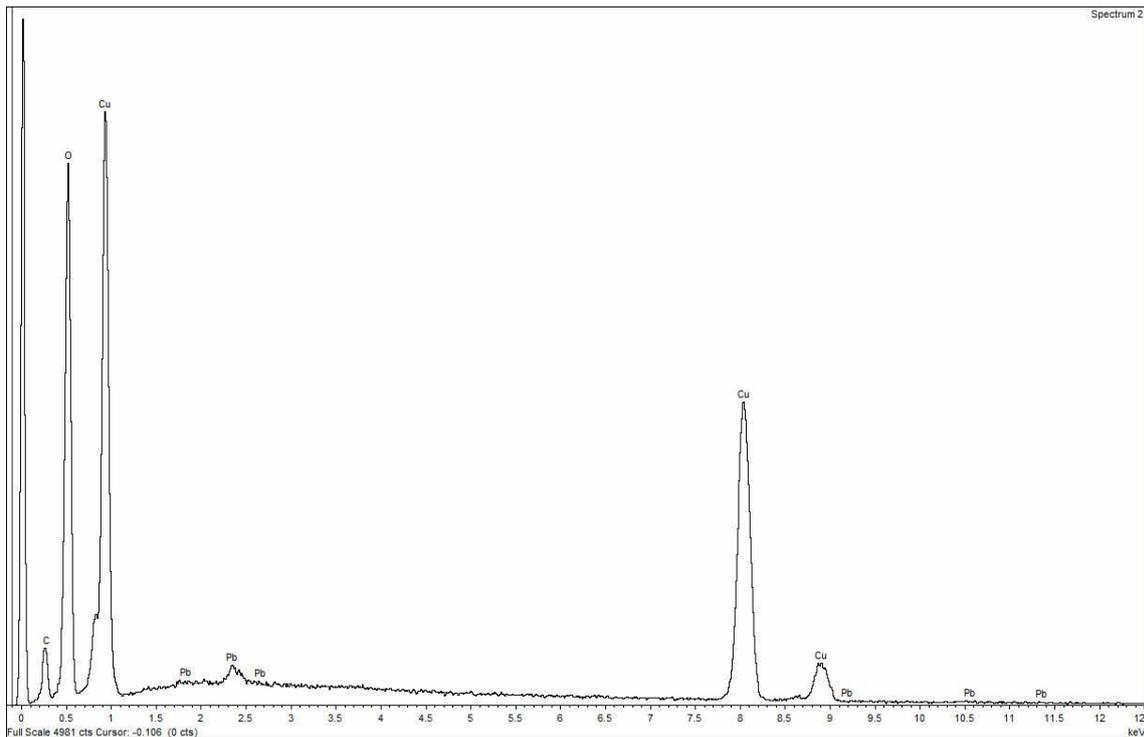
Figure 19. Typical SEM-EDS spectrum obtained in the copper carbonate grains in a polished cross-section of the green material from K355.
