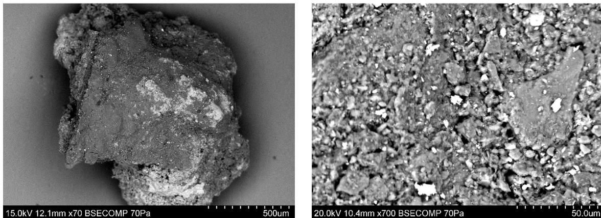
*Figure 21. Overall view of sample from K680 under the SEM (left), and detail of its surface, showing clay minerals and some bright silver sulphides.*
