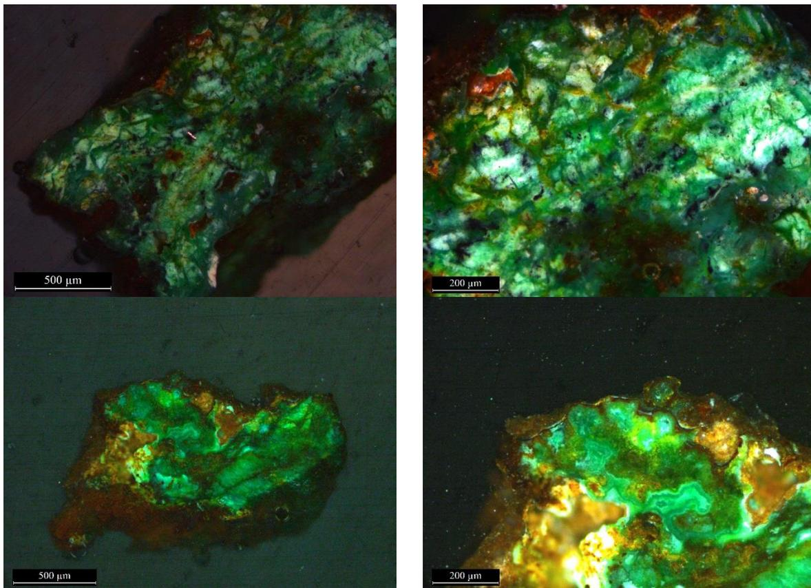
Figure 14. Four views of polished cross-sections of green material from K355, showing the predominance of green copper carbonates, together with some iron- and copper-rich red phases.
