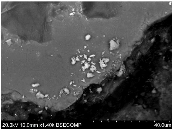
Figure 24. Detail of small bright crystals on the red particle in K572, as seen under the SEM.
