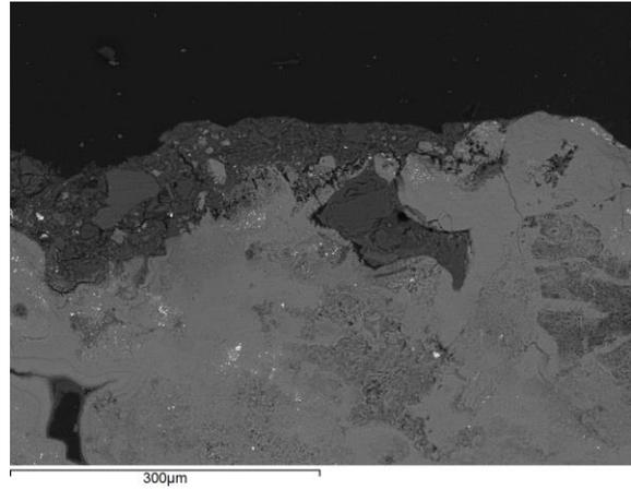
*Figure 16. SEM image of a cross-section sample from K355 showing an enrichment in soil contamination (darker grey) towards the surface.*
