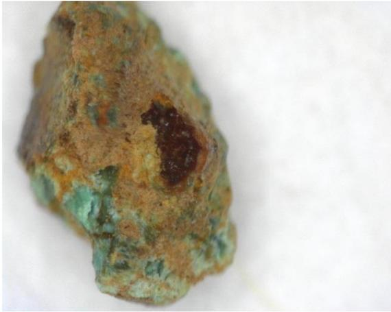
Figure 22. Sample from K572 under the digital microscope, showing a red particle preserved in the porous mass of green and brown minerals. Figure 22.
