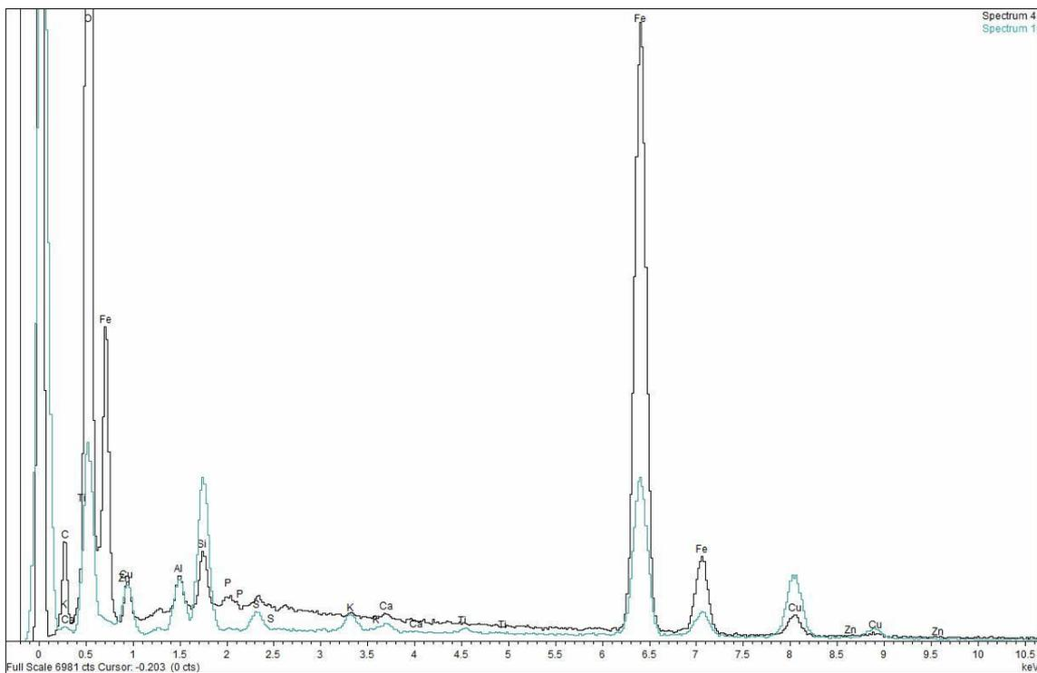
Figure 26. Comparison of SEM-EDS spectra for the red particle (black line) and the adjacent matrix (blue line), as shown in Figures 22 and 23.
