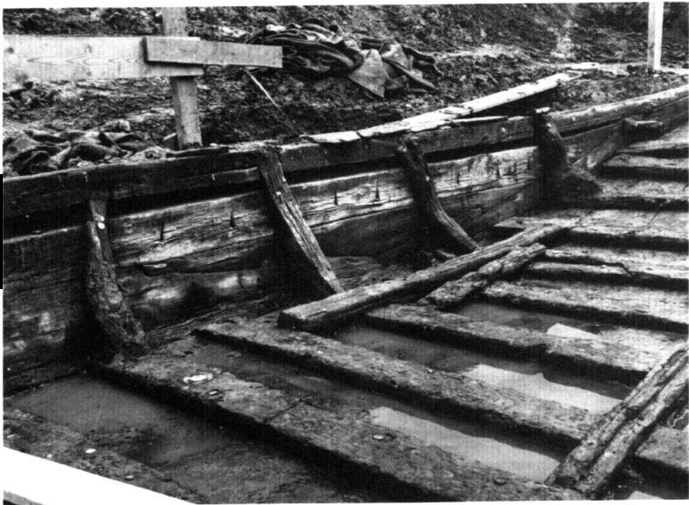
Fig 23 Ferry-like barge Zwammerdam 6: part of the bottom and a side. Knee-ended ribs are placed in alternate positions. A double-hooked plank is used to brace the rising end-sections (photo IPP: G Verkuil)
