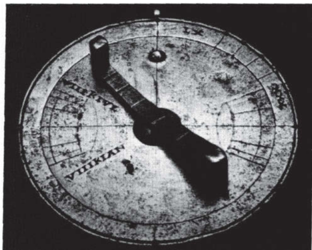
Fig 14 Portable sundial in the Oxford Museum of the History of Science, probably 3rd century AD. This type was designed for use at all latitudes, and has those of many provinces inscribed on the reverse (Britain is at 57°)
