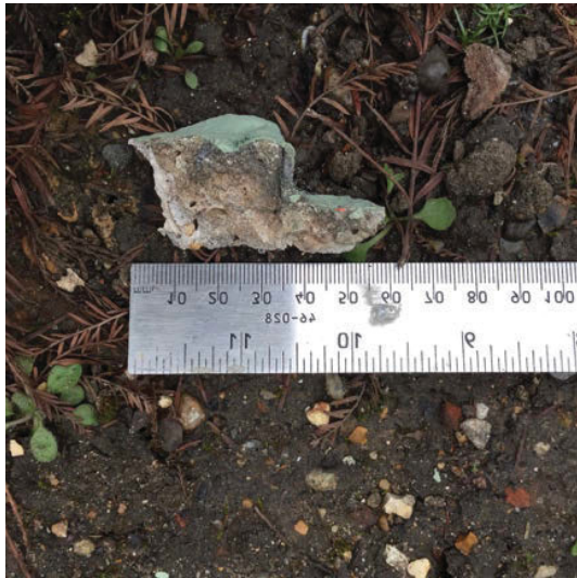
Plate 5. Photographed 10.03.17 - Disassociated fragment from point 540mm along crack 1A
