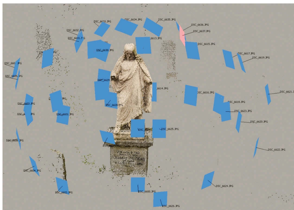
Plate 19. Screen shot showing the position of the camera used to create the digital image of the sculpture using photogrammetry 18 .
