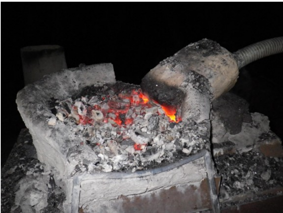
An experimental approach to studying bloom refining - a bloom remelting experiment run with friends in Virginia
