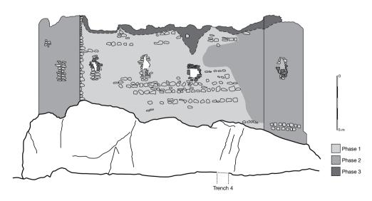
ILLUS 3 Interpretative south-west elevation showing the general architectural sequencing of the castle's structural development. The earliest surviving phase consisted of the central part of the wall characterised by the lancet windows and large facing stones. Corner towers were later added while larger windows and gun loops were added in the late medieval period. In the 18th century additional refurbishment of the parapet took place
