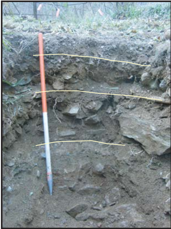
Plate 1: Detail of the section through the evaluation trench with the road layers highlighted
