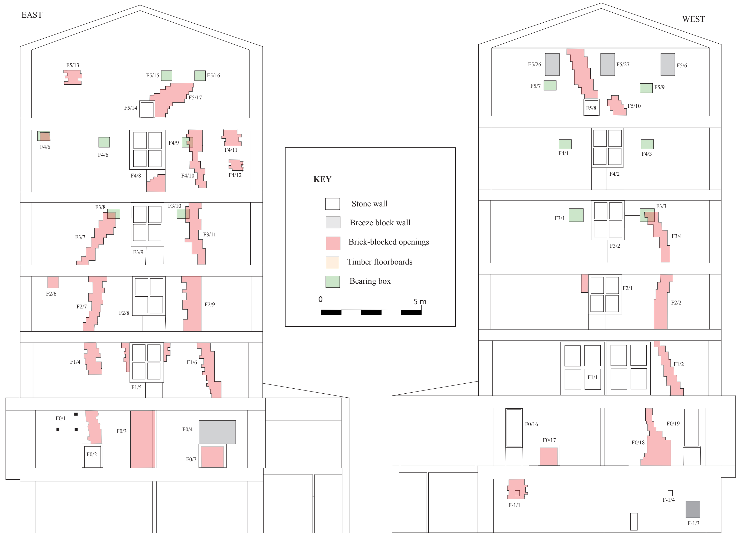
Figure 26: Cross section showing the features on the internal face of the end walls
