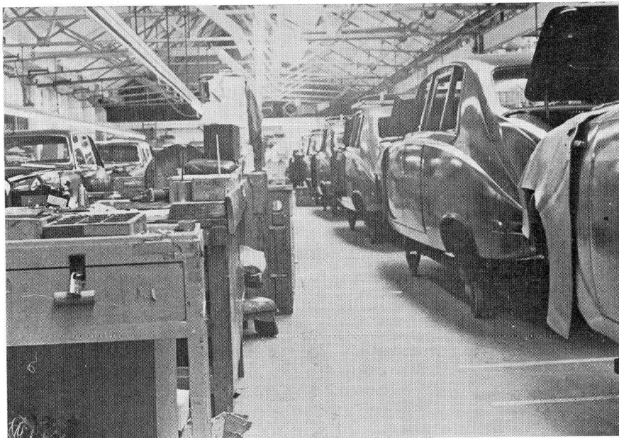
Fig. 1: Vanden Plas coach-building line at Kingsbury factory, showing limousine assembly. Note the trollies on which the car bodies are mounted during the early stages. These are guided by a wooden rail along the floor (not visible) — an early form of assembly line? Note also the leather protective covers draped over the wings whilst work is done on the engine compartment. (photo: David Thompson)
