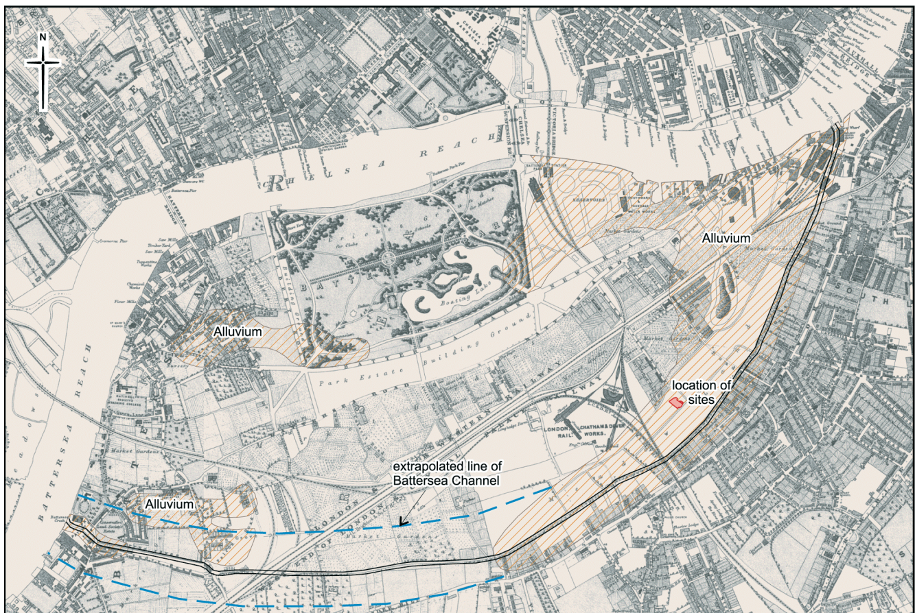
Fig. 3: extract from Stanford's 1862 map showing route of the 'sewer' which is now borough boundary between Wandsworth and Lambeth. Also shown is BGS mapped alluvium, and extrapolated possible course of the Battersea Channel
