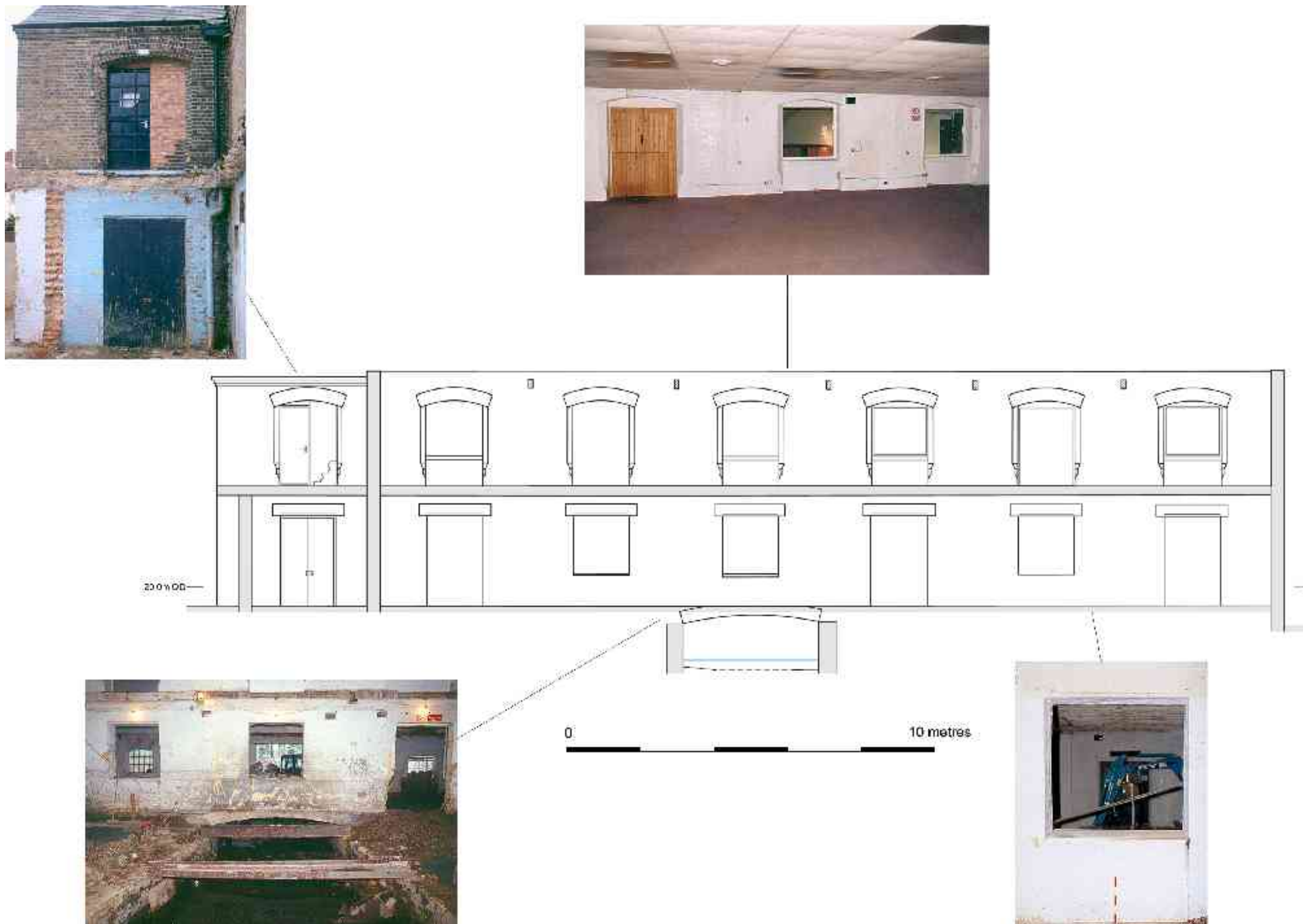
Fig 7 Elevation and views of the west face of the 1860s Grove Mill, now forming the central wall within the extended building. The photo at lower left shows the exposed millrace after removal of the floor slab
