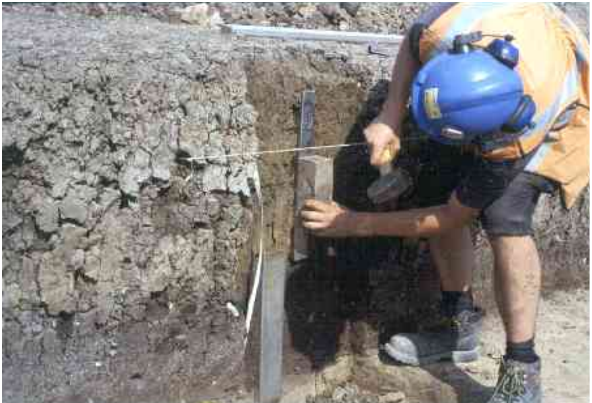
Fig 23 A member of the Museum of London Specialist Services hammering a monolith sampling tin into section I-J, towards the north-east corner of the excavation (Fig 9)
