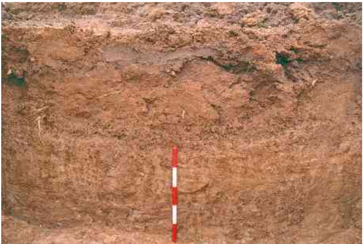
Fig 6 Detail of the exposed section seen in the foreground of Figure 5. A shallow layer of disturbed subsoil overlies natural: the latter changes from firm sandy silt to a lighter, much more sandy deposit at c 36.4m OD (approx. the top of the 0.5m scale)
