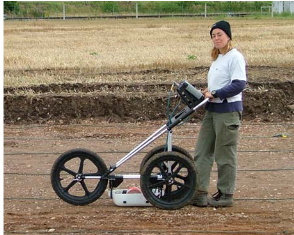
Figure 23. The SIR3000 GPR unit was used with a shielded 400 MHz antenna.
