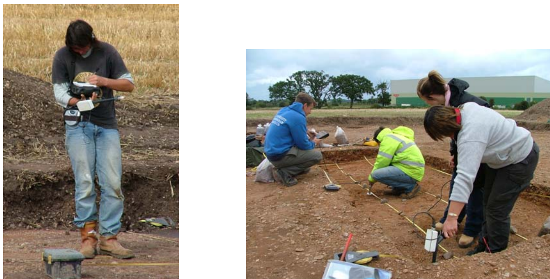
Figure 20. Magnetic Susceptibility data were collected with the Bartington MS2 susceptibility meter.
