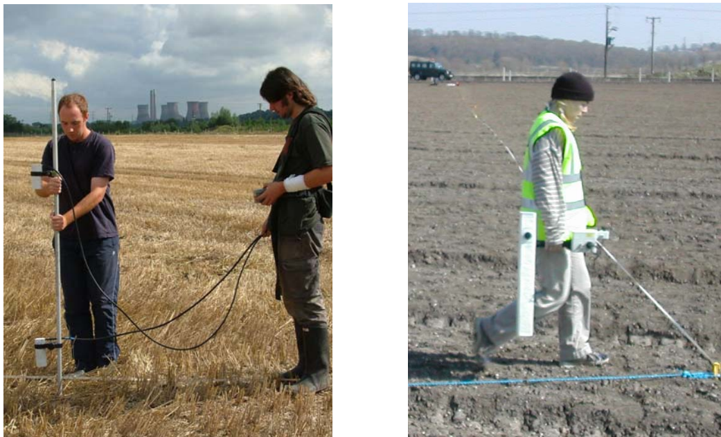
Figure 19. G858 Cesium Vapor magnetometer (right) in vertical gradient mode and the FM256 Fluxgate Gradiometer (left).
