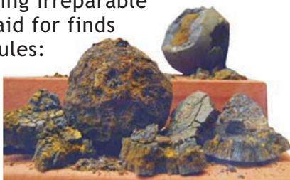
A Mary Rose Trust experiment demonstrates damage to cannonballs caused by improper conservation
