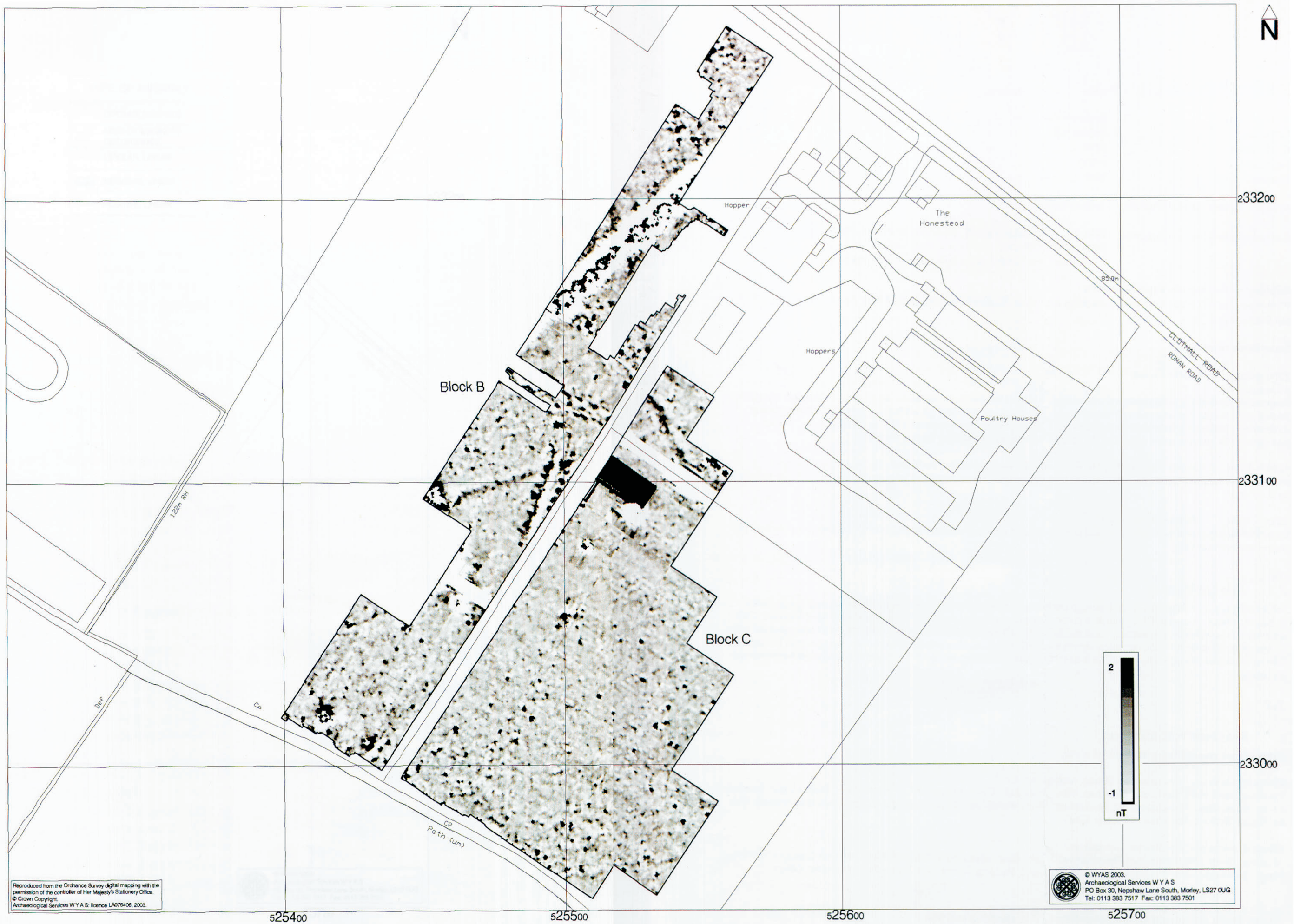
Fig. 5 Greyscale plot of gradiometer data; Blocks B and C
