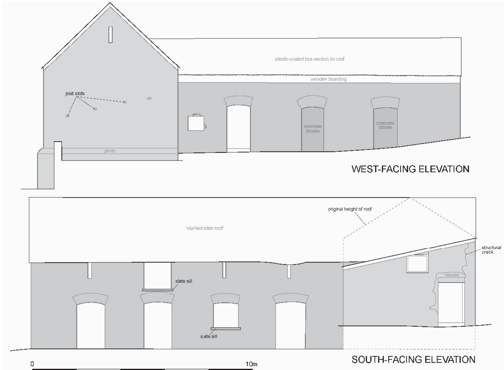
Figure 35: The west- and south-facing elevations of the Shippon complex.
