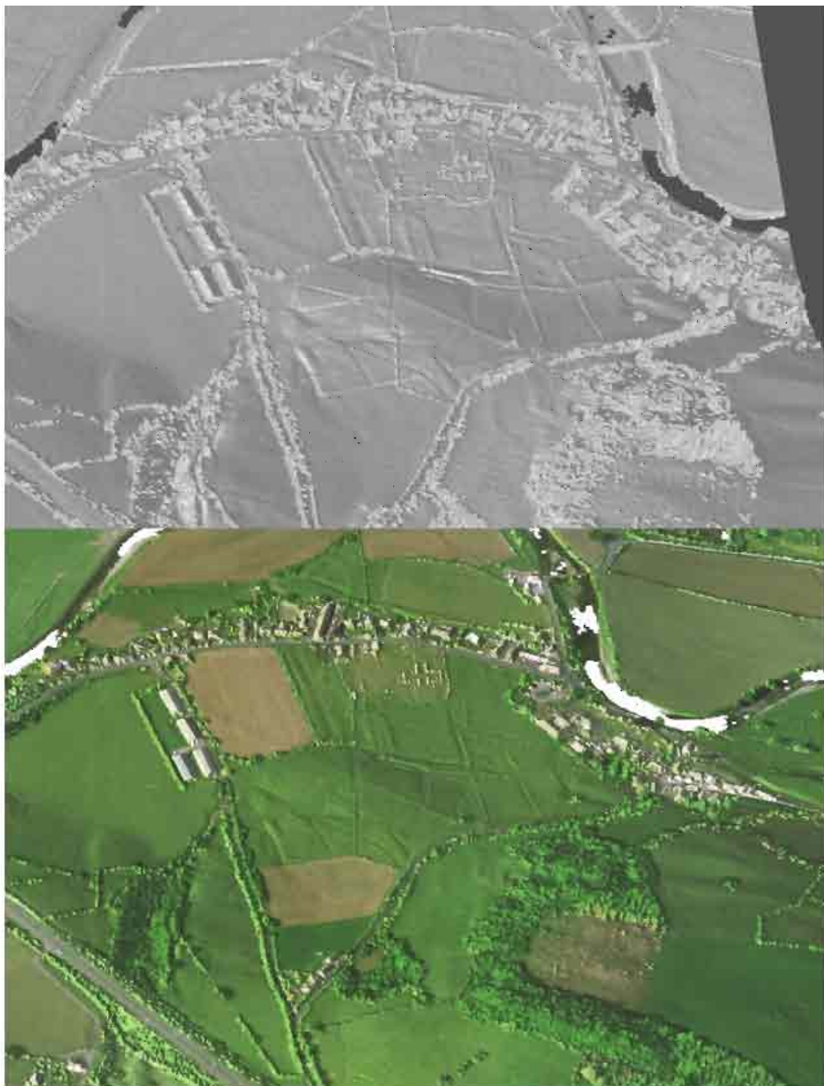
Figure 55: (Above) slope model of Sawley earthworks; (Below) vertical colour air photograph enhanced using LiDAR to create an oblique effect
