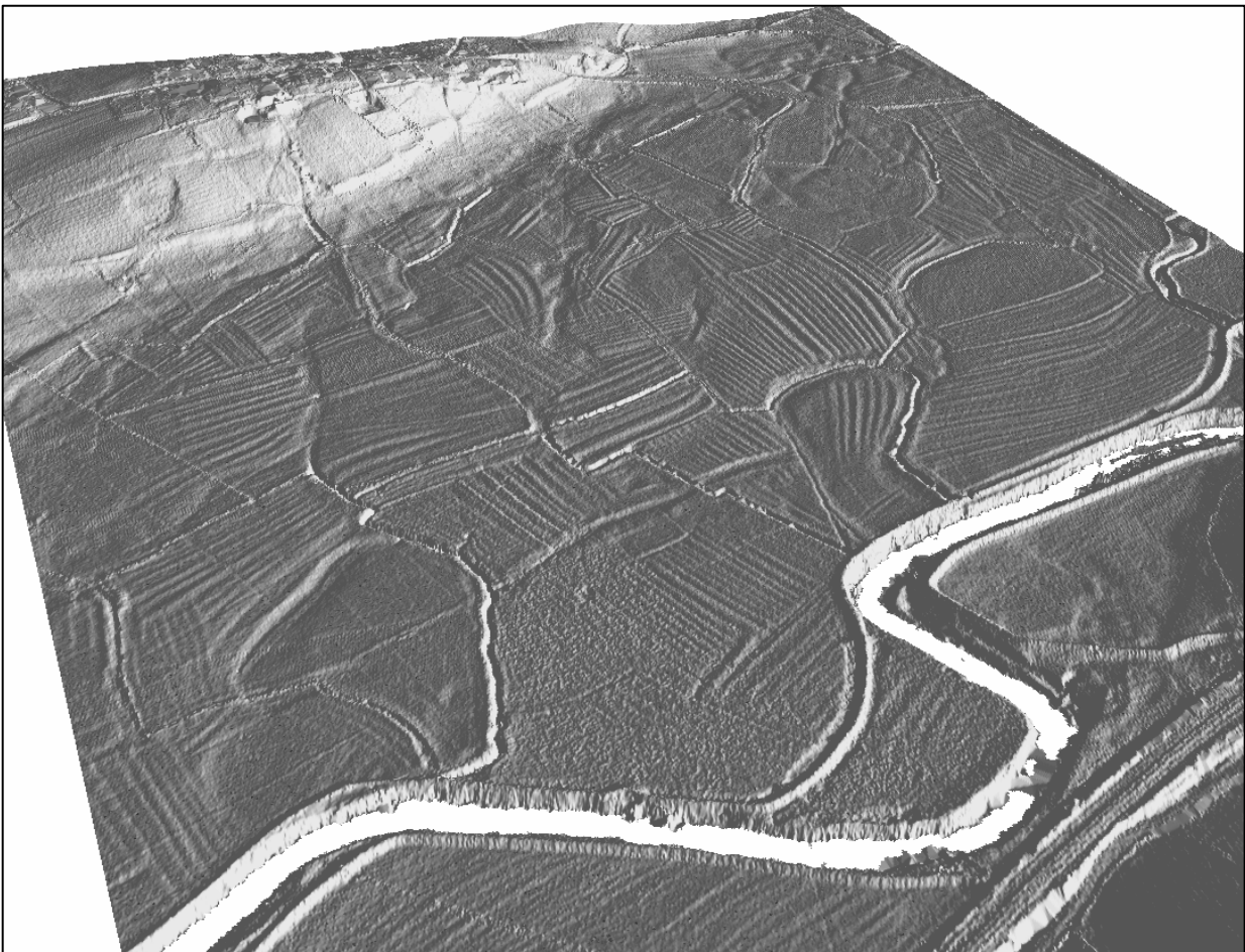
Figure 56: (Above) aerial photograph of ridge and furrow at Rathmel, North Yorkshire; (Below) LiDAR slope model displayed in ArcScene used to bring out additional detail
