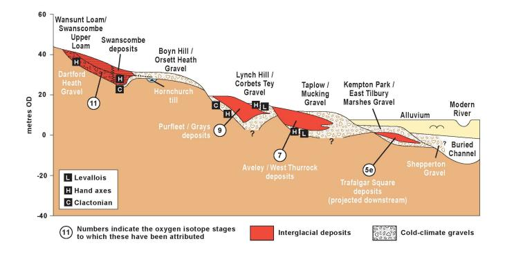
Fig 7 Geology: Lower Thames staircase diagram, transverse section with archaeology
