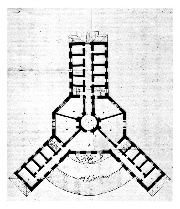
Fig. 1. Plan of the new House of Correction at Abingdon.
