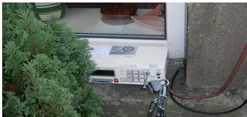
Figure 35: Grimm optical particle counter deployed at 2 West View Terrace, Horton in Ribblesdale.
