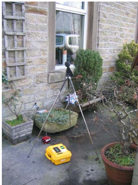
Figure 36: Sound intensity logger and geophone unit outside 2 West View
