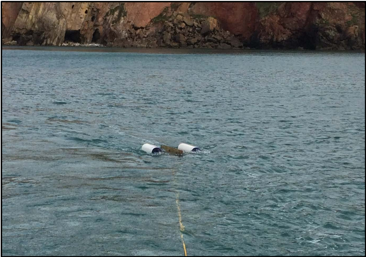
Figure 4: Magnetometer and float arrangement towed behind the vessel
