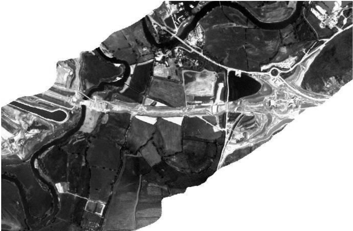
Figure 4. An example of geocorrected CASI data showing the distortion in the image data.
