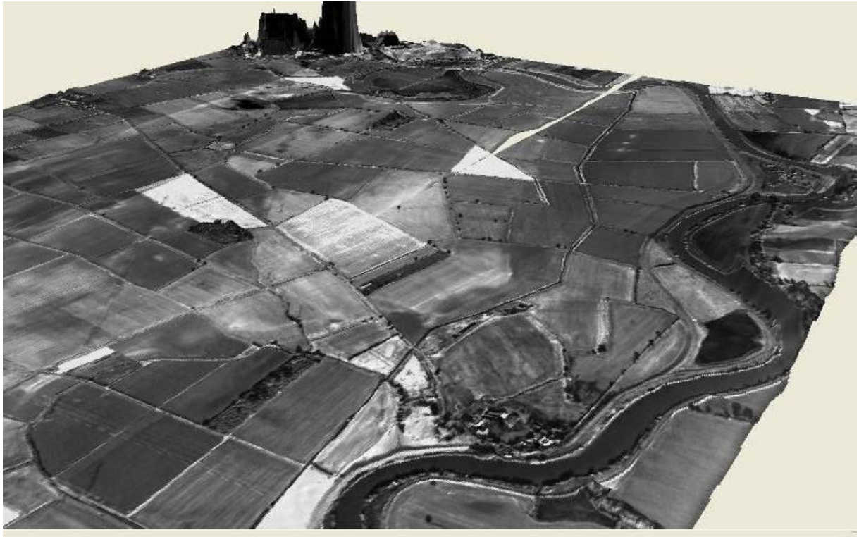
Figure 58. Eagle Principal Component 2 draped over the lidar DSM. In combination these data effectively highlight the terrace edge.
