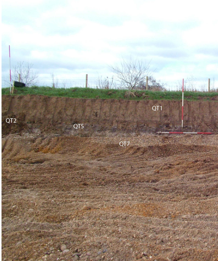
Fig 5.19: A photograph of the start of the T1QT transect, showing the main units from the GPR interpretation.
