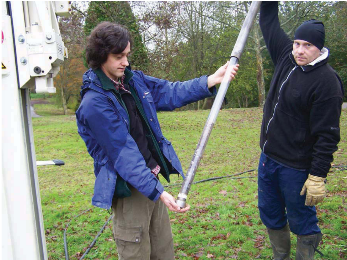
Fig 3.2: A sample recovered from the Geoprobe. The sample collection tube is shown coming out of the closed metal sampling chamber. The sample collection tubes used for OSL sampling were black opaque tubes.
