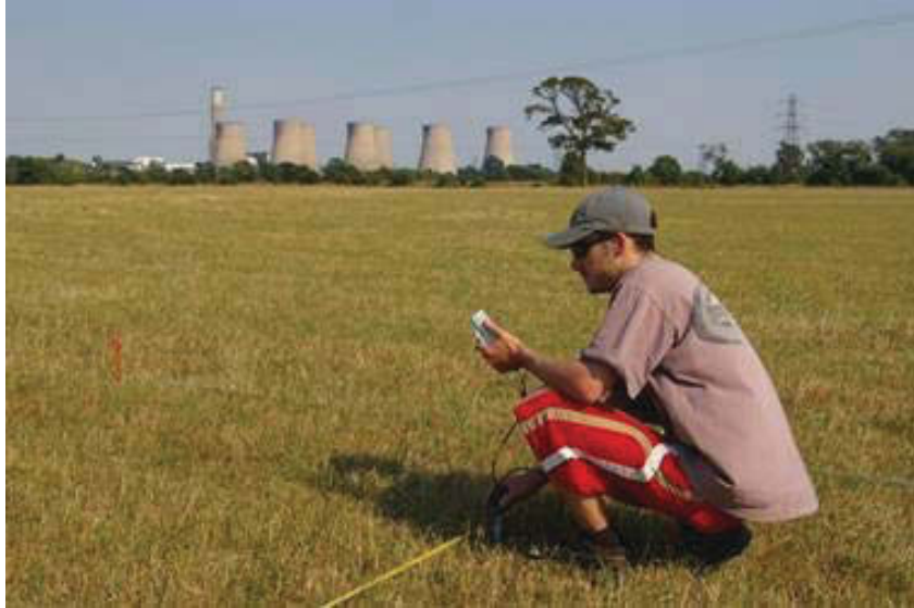
Fig 3.24: Lockington. Field collection of volumetric soil moisture data at regular grid intervals using a Delta T Devices Theta Probe.
