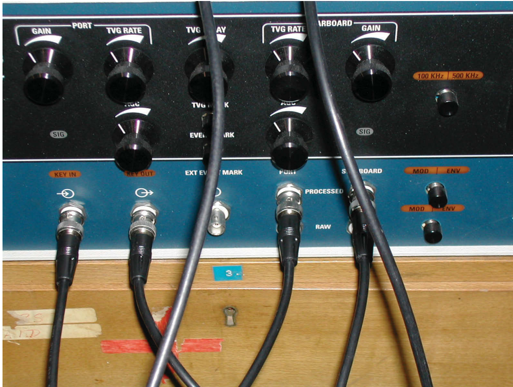
Fig. A-46. Front connection panel of side-scan deck unit. If the processed data is being recorded, the gains, TVG and AGC controls will need to be adjusted.
