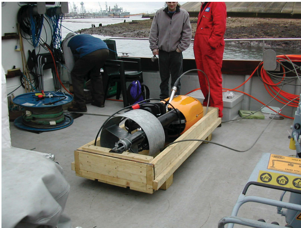
Fig. A-40. Dual profiler fish in case during mobilisation. Large fin acts as stabilizer.
