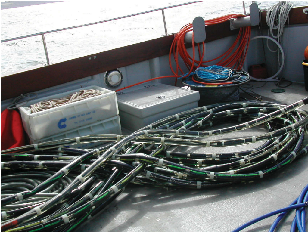
Fig. A-53. Streamer flaked on Xplorer back deck.
