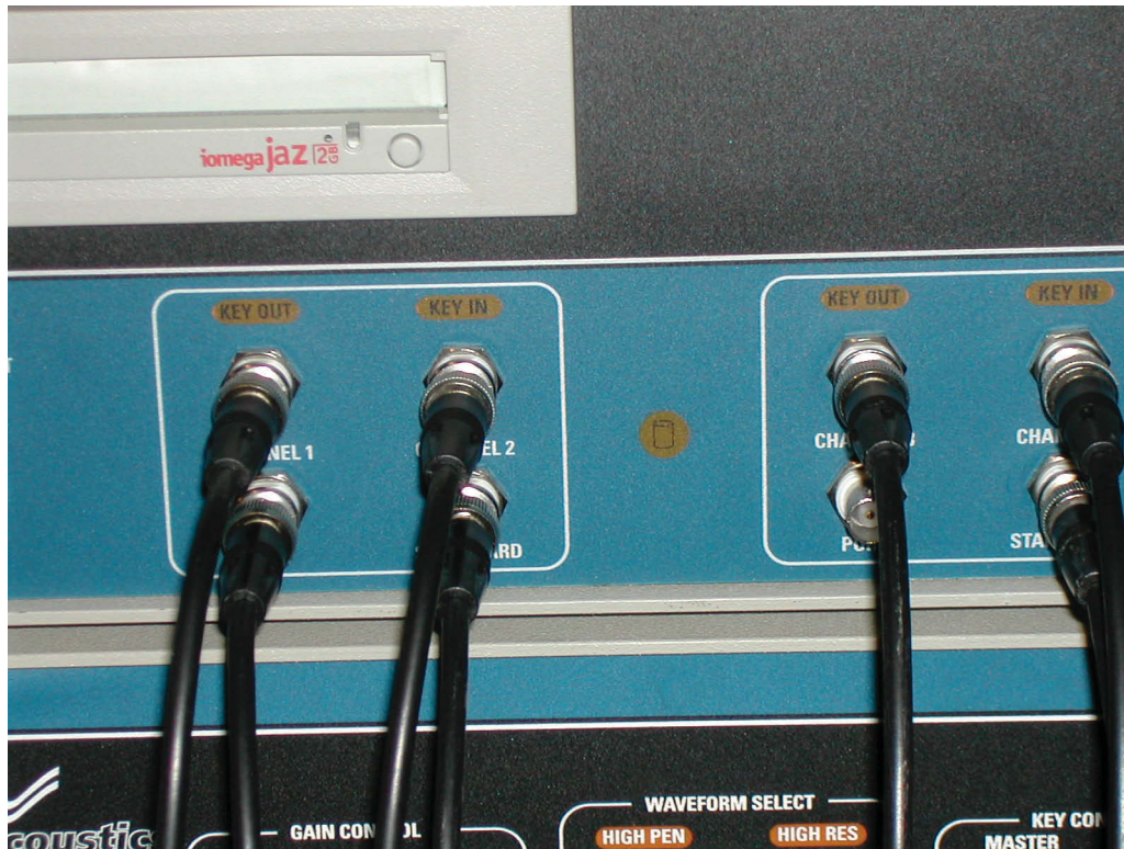
Fig. A-44. Front connection panel of GeoPro computer.
