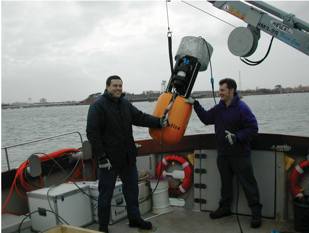
Fig. A-41. Dual profiler fish prior to deployment. Yellow fibreglass case contains the four chirp transducers, with the side-scan sonar transducers along the side. Fish is ‘head heavy’ due to lead weights to aid level buoyancy in water during survey.
