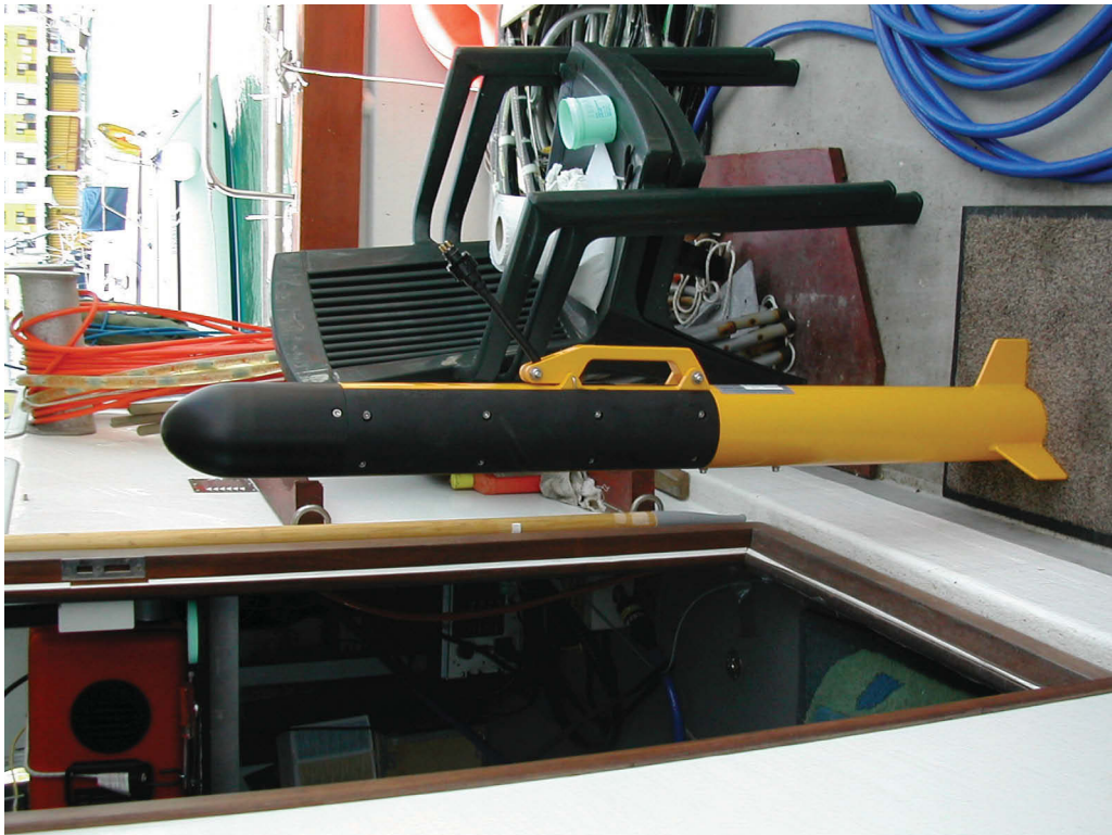
Fig. A-42. Small, side-scan only fish. Torpedo shape allows for better ‘flying’ and easier deployment/recovery.
