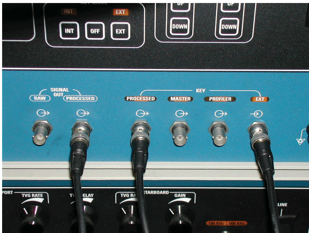
Fig. A-45. Front connection panel of Chirp deck unit. Signal out, contains the data going into the acquisition computer. The two key connections relay the fire from the software and when to record the hydrophone data.
