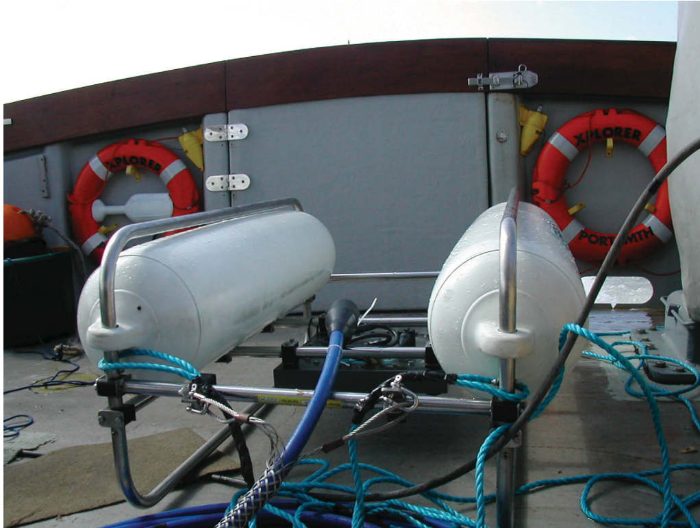
Fig. A-52. Catamaran with boomer plate in the centre. Blue cable is the HV as indicated in Fig. A-51.
