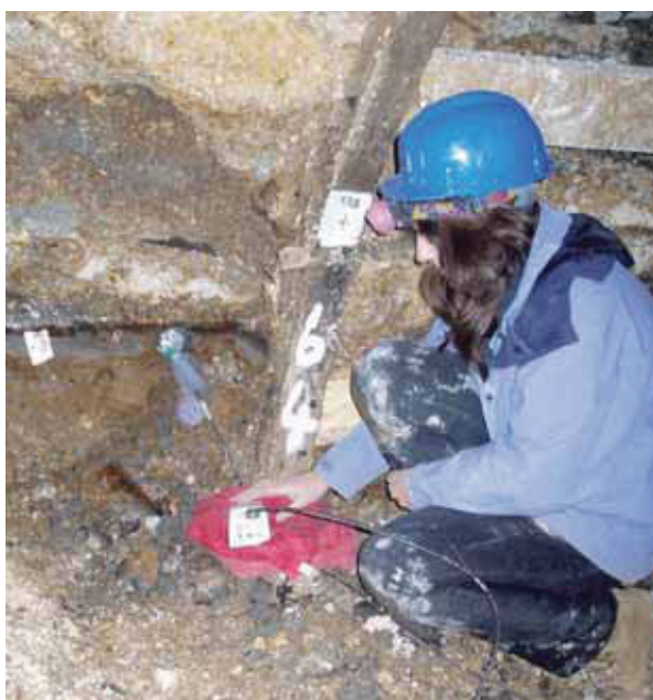
Fig 26 (above) Measurement was undertaken for one hour and produced the energy spectrum shown (peaks used to estimate K, U and Th concentrations are marked – the energy peak of 1460keV from K is particularly prominent). (left) A portable gamma spectrometer being used to make an in situ measurement of the gamma dose rate for a sample collected from a buried surface preserved within Silbury Hill, Wiltshire.
