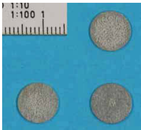
Fig 18 Aliquots for luminescence measurements may contain different numbers of grains: each metal sample disc is 9.8mm diam; changing the proportion of the disc surface used varies the number of quartz grains (c 0.2mm diam) (upper right c 1000 grains, bottom left c 200, bottom right c 20) (photograph by H Rodnight).
