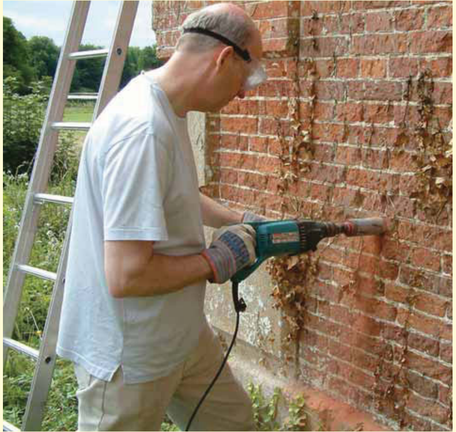
Fig 40 Using a diamond tipped drill barrel to sample a brick for OSL dating.
