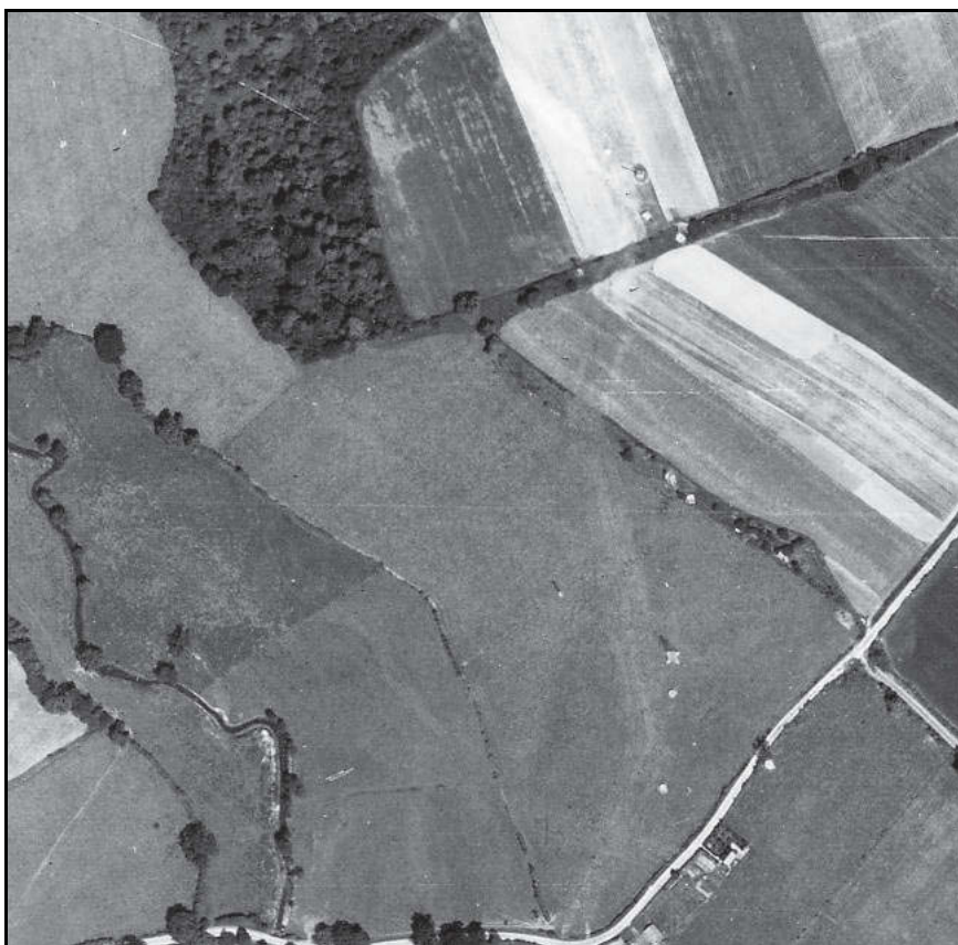
Figure 58. The GHQ Line A to the south of Heckfield, Blackwater catchment. The line of the anti-tank ditch runs in a zigzag pattern through the fields from north to south. There are pillboxes hidden in field hedges to the east. Photo: RAF 106G/UK/1647/2019. 11-JUL-1946. English Heritage. NMR (RAF Photography)
