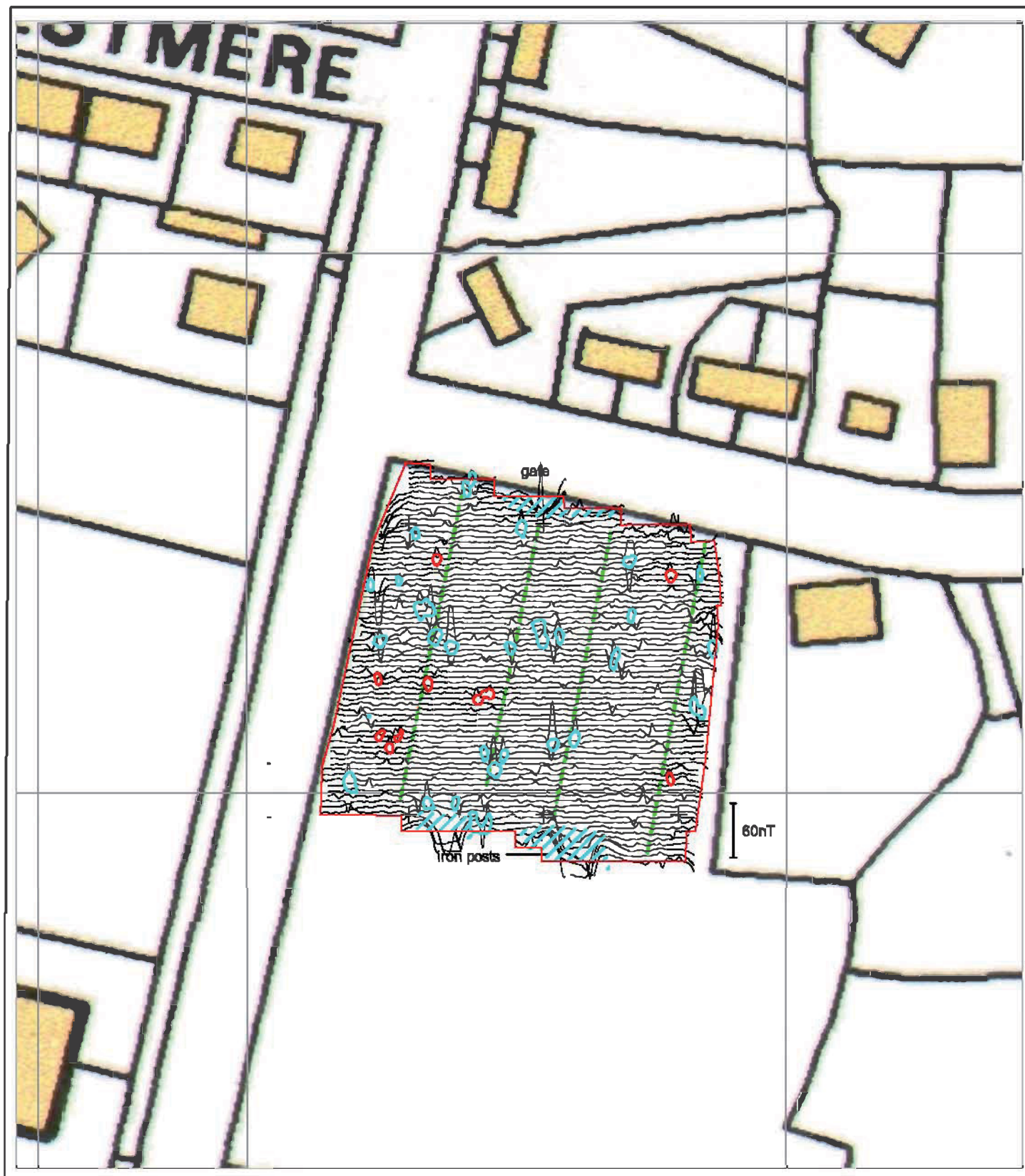
HANLEY SWAN, WORCESTERSHIRE Geophysical Survey 2009 Figure 3: Magnetometer survey (with interpretation)
