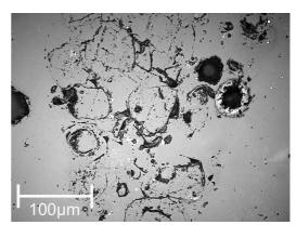
**Sample:** Blast furnace slag – Sowerby Bridge SOW-K
