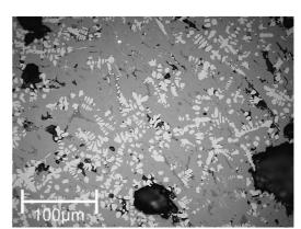
**Sample:** Iron smelting slag – Myers Wood B210s-I
