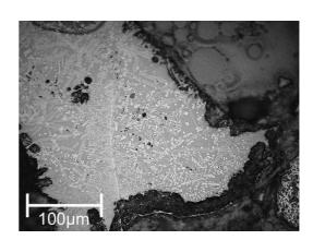
**Sample:** Blast furnace slag – Bretton BRE-F
