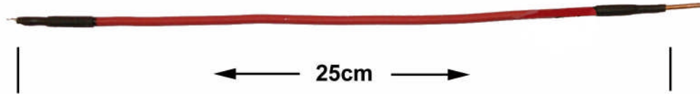
Figure 4.3: Close-up of redox probe: left terminal has 'welded' platinum wire tip, red and black = shrink-fit sleeve, right end has copper wire exposed for connection to pH\mV meter (© Malcolm Lillie).
