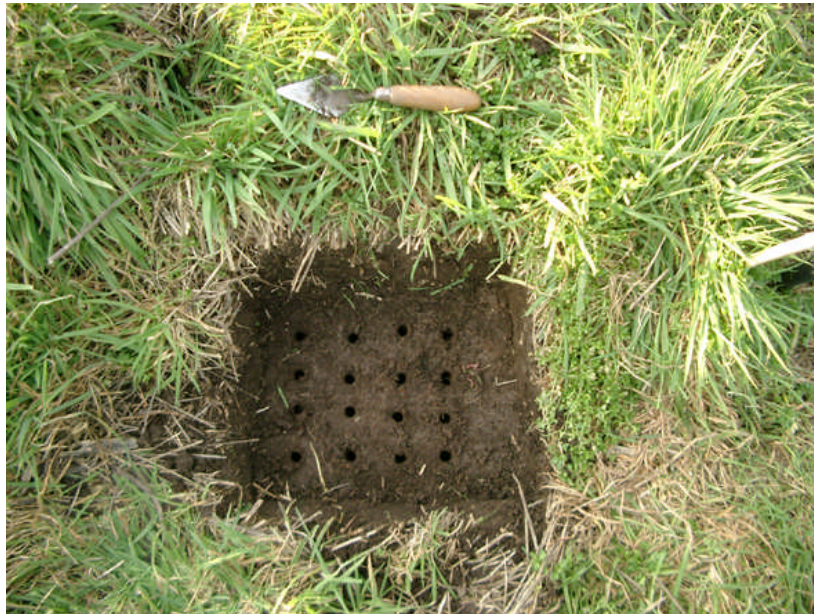
Plate 4.4: Augured holes for insertion of redox cluster, four holes were excavated to depths of 0.1m, 0.5m, 1.0m, and 2.0m depths, with four replicate probes at each depth (© Malcolm Lillie).
