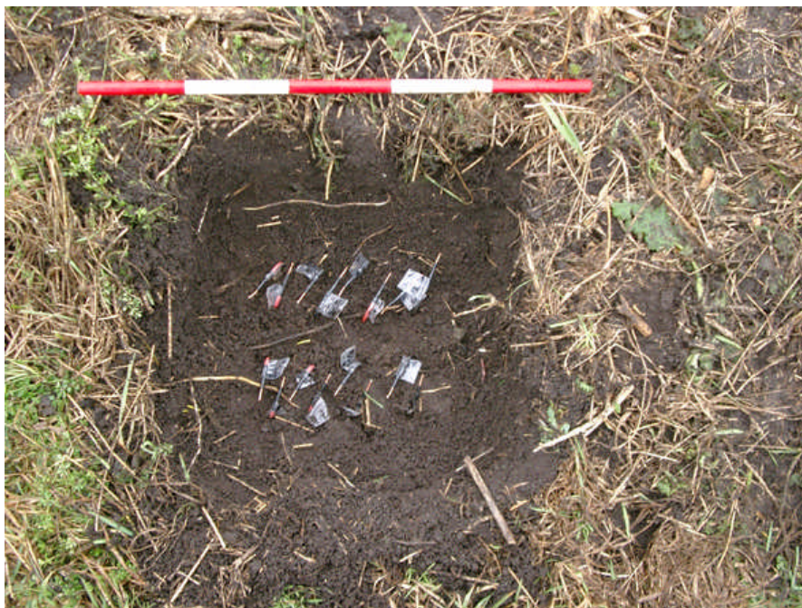
Plate 4.5: Redox probes after insertion to required depths (© Malcolm Lillie).
