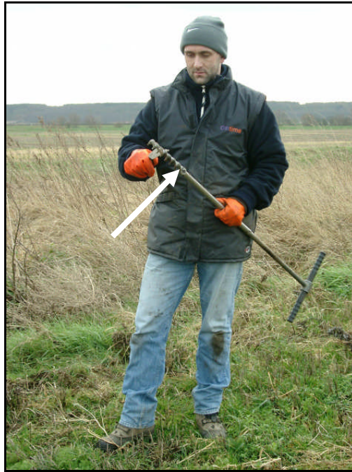
Plate 4.1: Close-up of 30mm diameter Van Walt screw tip augur used in piezometer installation (© Malcolm Lillie).
