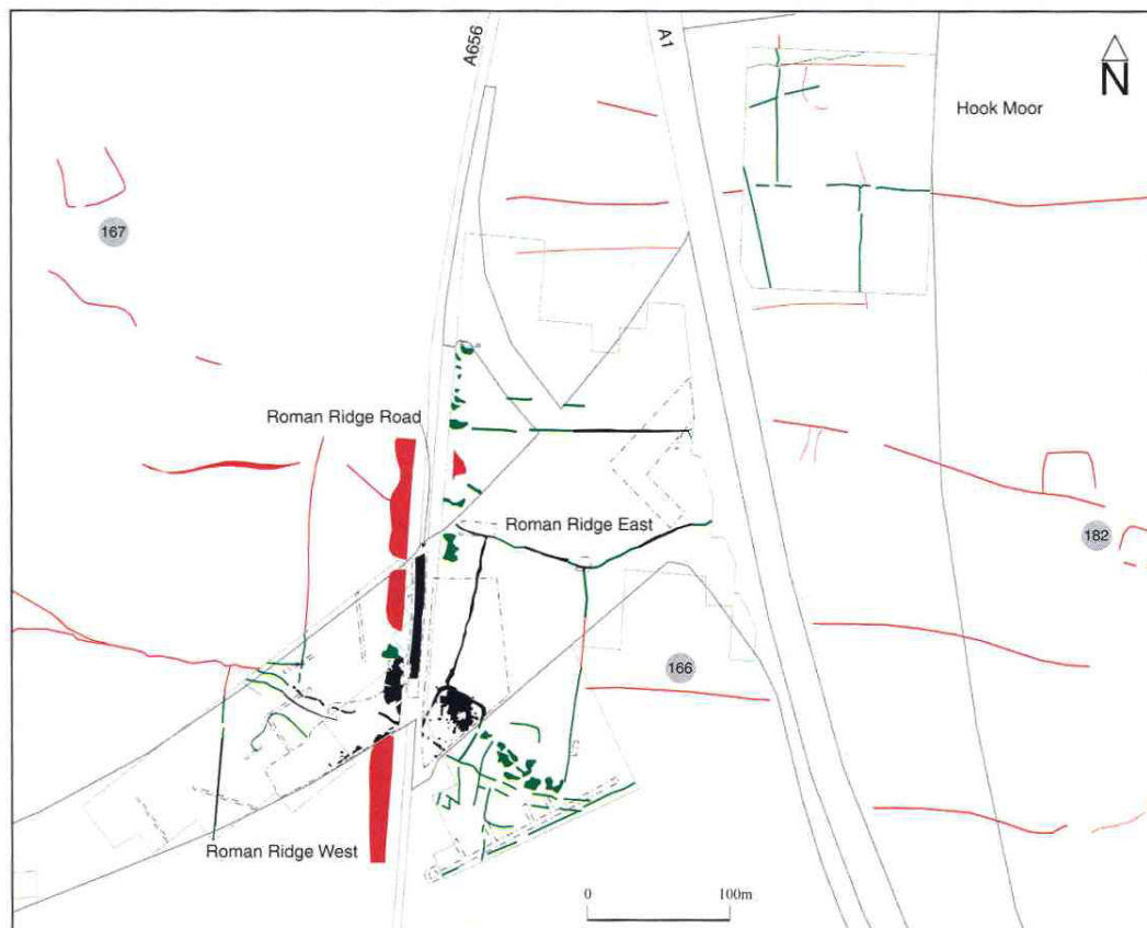
Figure 2.11. Investigation of the Roman road at Roman Ridge, West Yorkshire, showing the road (now the north-south line of the A658) cutting across pre-existing boundaries and enclosures. Excavated features in black, geophysical survey results in green, and cropmarks in red. (Source: Deegan 2001b: 33, fig. 17).
