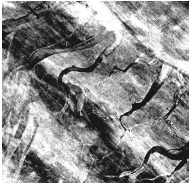
Figure 6: Shallow time slice from HD3D data in Qatar. The resolution of the complex meandering channel systems is outstanding, and signal-to-noise quality is a step improvement over historical seismic data in such shallow waters. Data courtesy of Maersk Petroleum (Qatar) Ltd.
