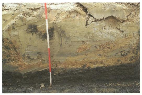
PI. 5 Sample section of deposit in foul pipe trench 8m south west of the most south easterly manhole, looking north west.
