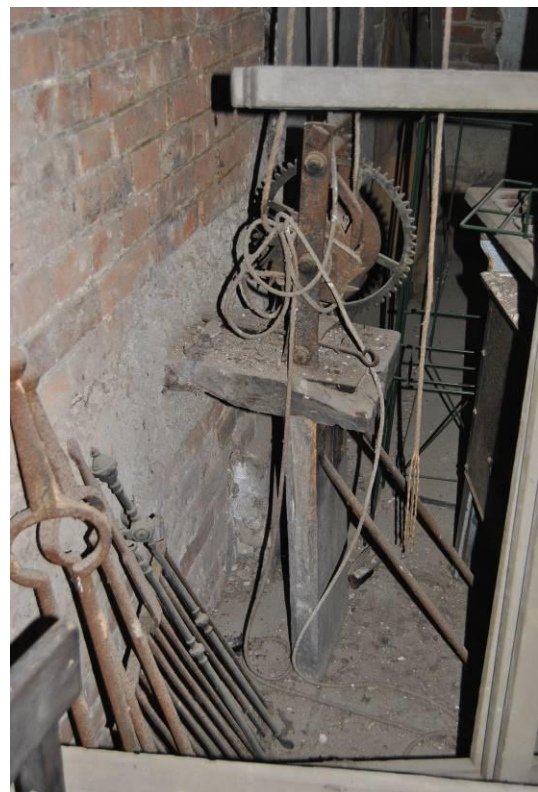
Plate 70: Winding gear for ceiling mounted airers.
