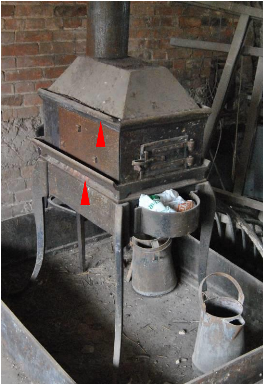
Plate 67: Laundry stove with profiled ledges (marked) for heating of flat-irons against chamber.
