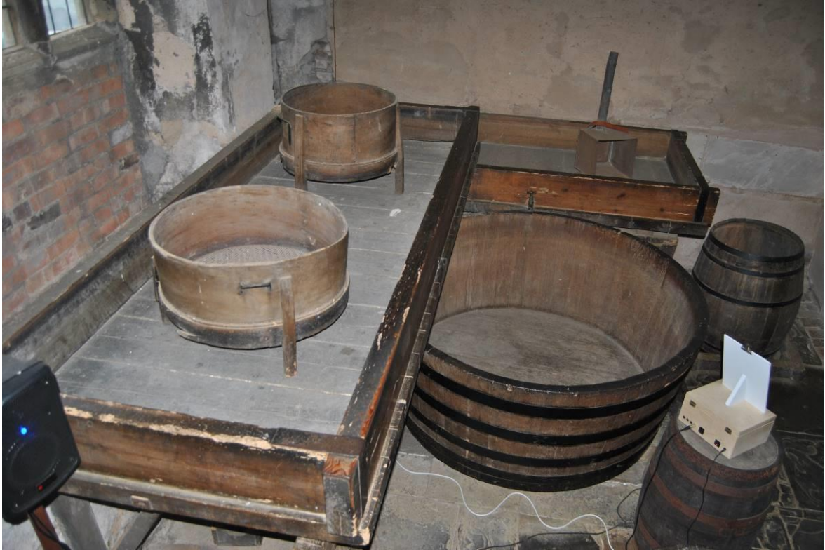
Plate 50: Paired timber coolers to north-east corner, fed from the northern copper, with fermenting tun beneath. NB. circular sieves within upper cooling tray for the straining of spent hops.
