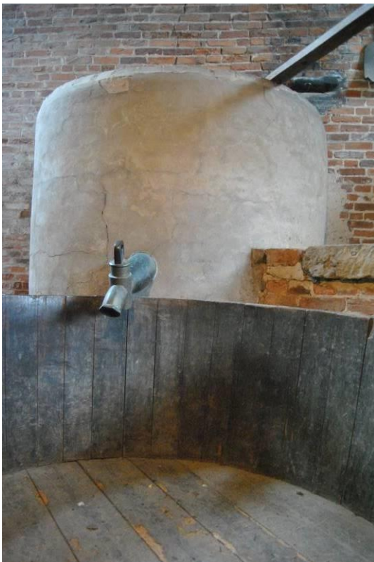
Plate 48: Copper feeding into mash tun.
