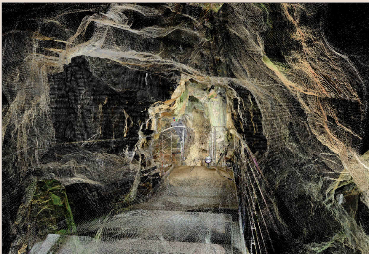
Fig.5.2. Laser technology provides a highly accurate and cost-effective tool for the surveying of subterranean features, as demonstrated by this unprocessed point cloud image of the interior of Church Hole cave. Photograph © Trent & Peak Archaeology
