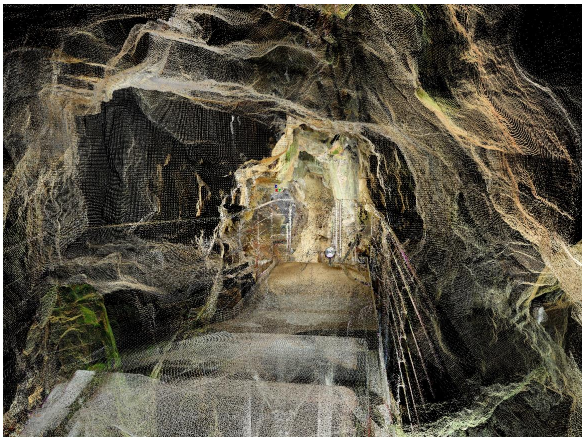
Fig.39. Laser technology provides a highly accurate and cost-effective tool for the surveying of subterranean features, as demonstrated by this unprocessed point cloud image of the interior of Church Hole Cave, Creswell Crags. © Trent & Peak Archaeology
