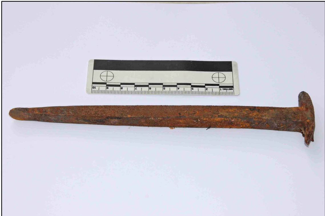
Appendix I.48: Large wrought-iron fixing nail from rafter (10cm scale) (Photo D175)
