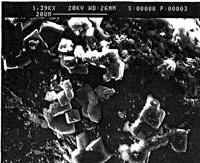
Plate 3 Detail of crystals, note cubic form (x1390)
