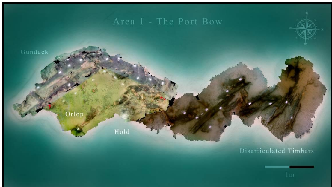
Figure 11: Image showing the original photogrammetry model of Area 1 with Photoscan targets. This image also identifies the three separate data sets, which have been merged to form Area 1 © PAS.
