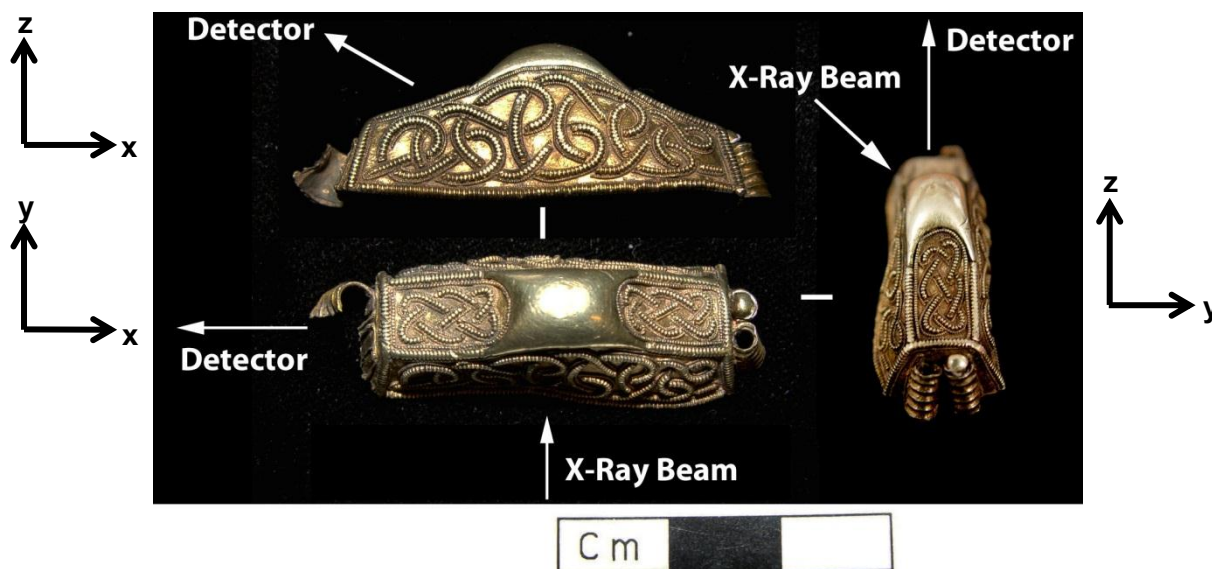
Figure 19. Photograph of the top and side of pommel cap K88 showing the spatial relationship between the object, the XRF detector and incident X-ray beam. The plane horizontal and vertical axes will be referred to as x-axis and y-axis respectively.
