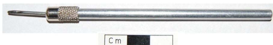
Figure 8. Tool used to scrape the surface to reveal the sub-surface.
