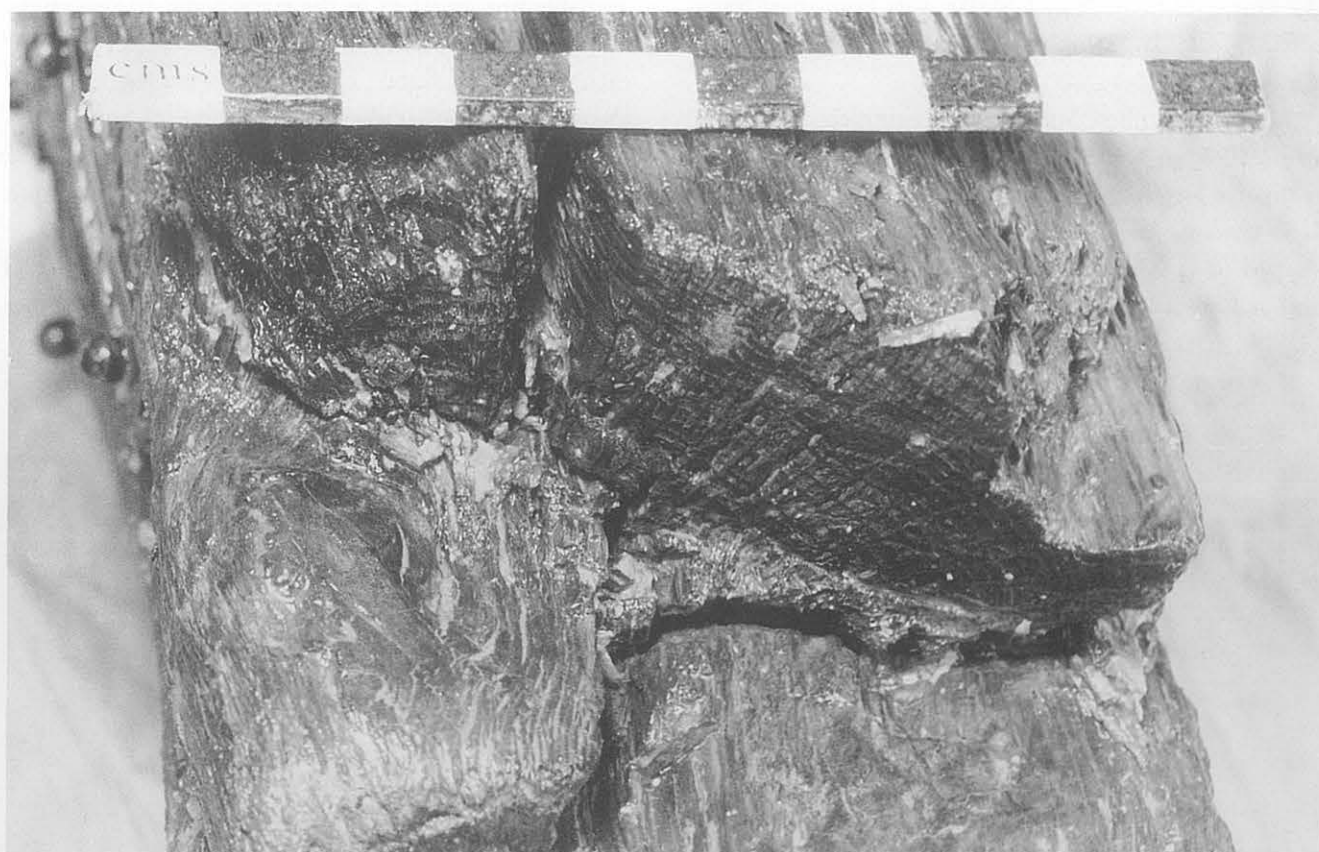
Figure 6.15 An angled groove cut into the after face of side timber SF6.5Pt towards its upper end. Inboard is to the right.
