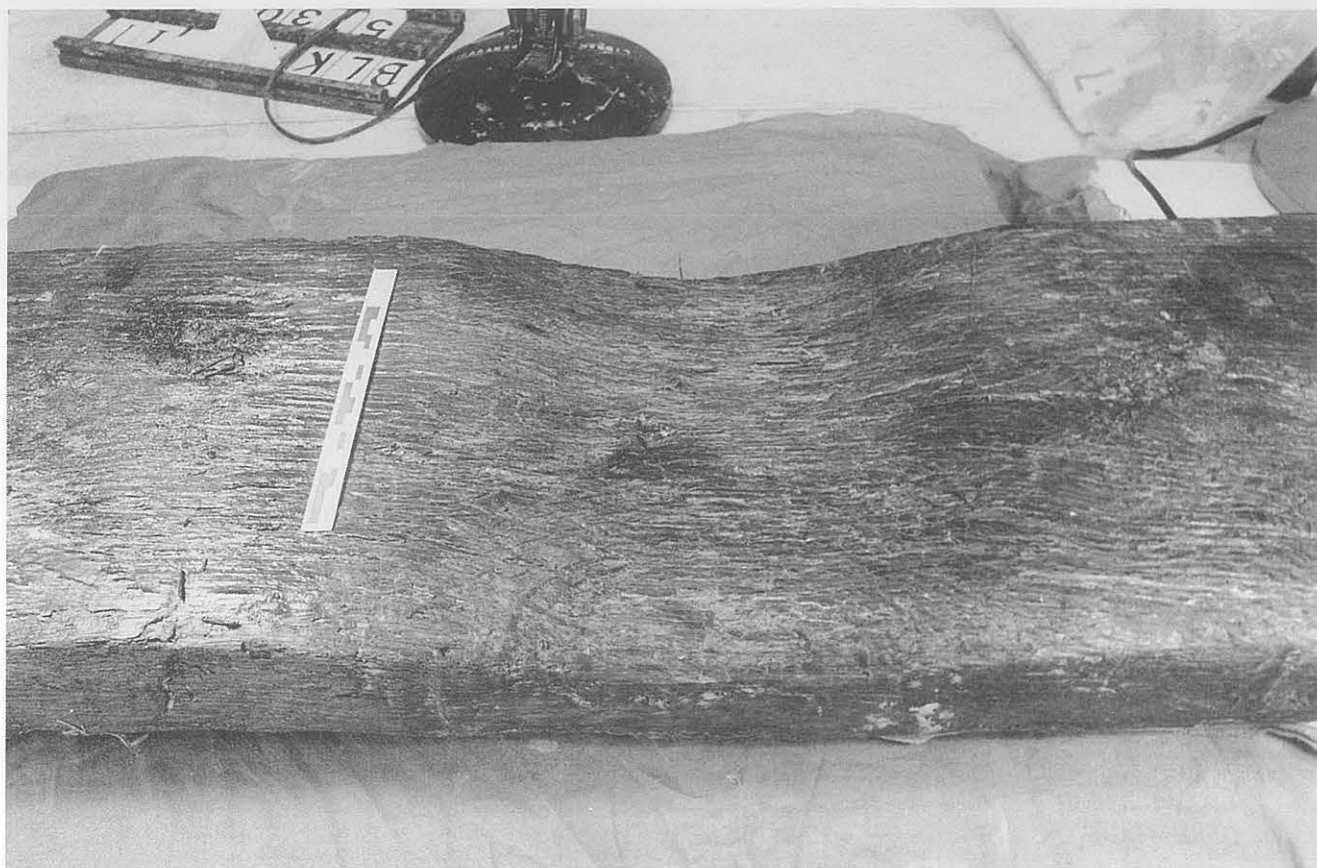
Figure 6.9A Worn area on plank-keel P1 between half-frame F5St and floor F6.
