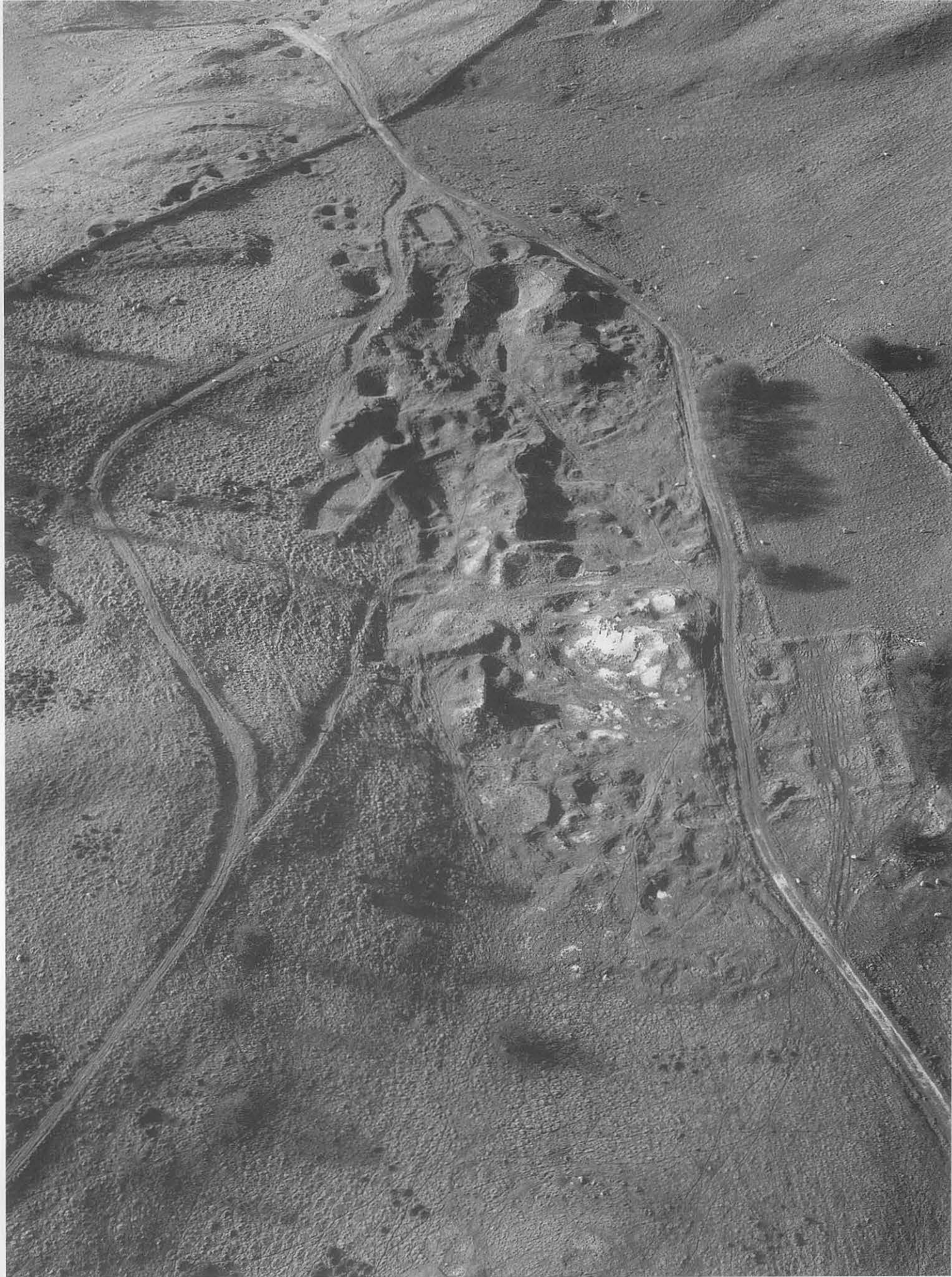
Figure 92 Aerial view of Belgrave mine from the south-east, showing the line of workings which run along the Belgrave vein across the hill to Bryn-yr-orsedd. (CPAT 90-MB-302)
