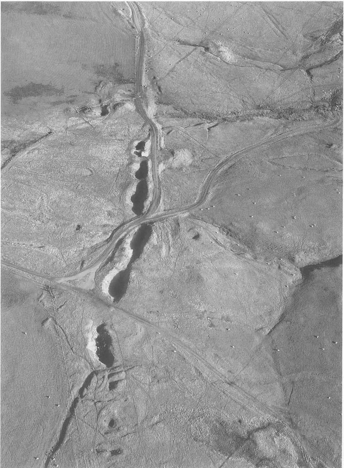
Figure 9 Aerial view of Pen Dylife mine, Llanbrynmair, Powys, from the west, showing a series of collapsed workings along the Pen Dylife vein. Many of these shafts have associated whim circles providing evidence for winding. (Crown Copyright: RCAHMW 925091-44)
