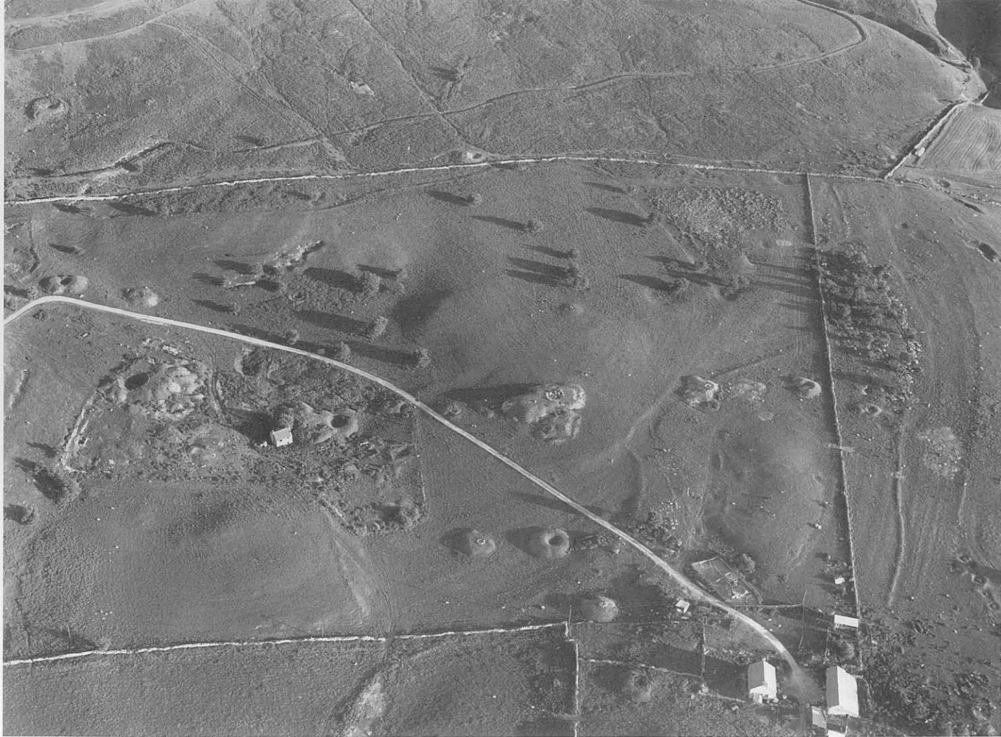
Figure 116 Aerial view of Lower Park mine, seen from the north-east with the farmhouse of Park Farm towards the lower right-hand corner. The main shaft, mine office and dressing floor in the walled enclosure just below the track to the right, with other shafts strung out along the Park vein. Part of a relict field system is visible beyond the farmhouse, towards the right-hand side. One of the notable features of the mine is a number of 19th-century beehive-capped shafts (to the left of the track in the foreground). A mining lease granted to Adam Eyton, a lead smelter from Llanerch-y-mor and Edward Williams of Wrexham by the duke of Westminster in December 1882 stipulated that they should build a 'substantial stone wall around pits ... when the pit goes out of use' and then 'fill up with earth and waste and cover with arch of stone'. The main period of working was between the 1820s and 1860s, before Hill Shaft and New Shaft were sunk further east along the vein on Esclusham in the 1860s and 1870s.
