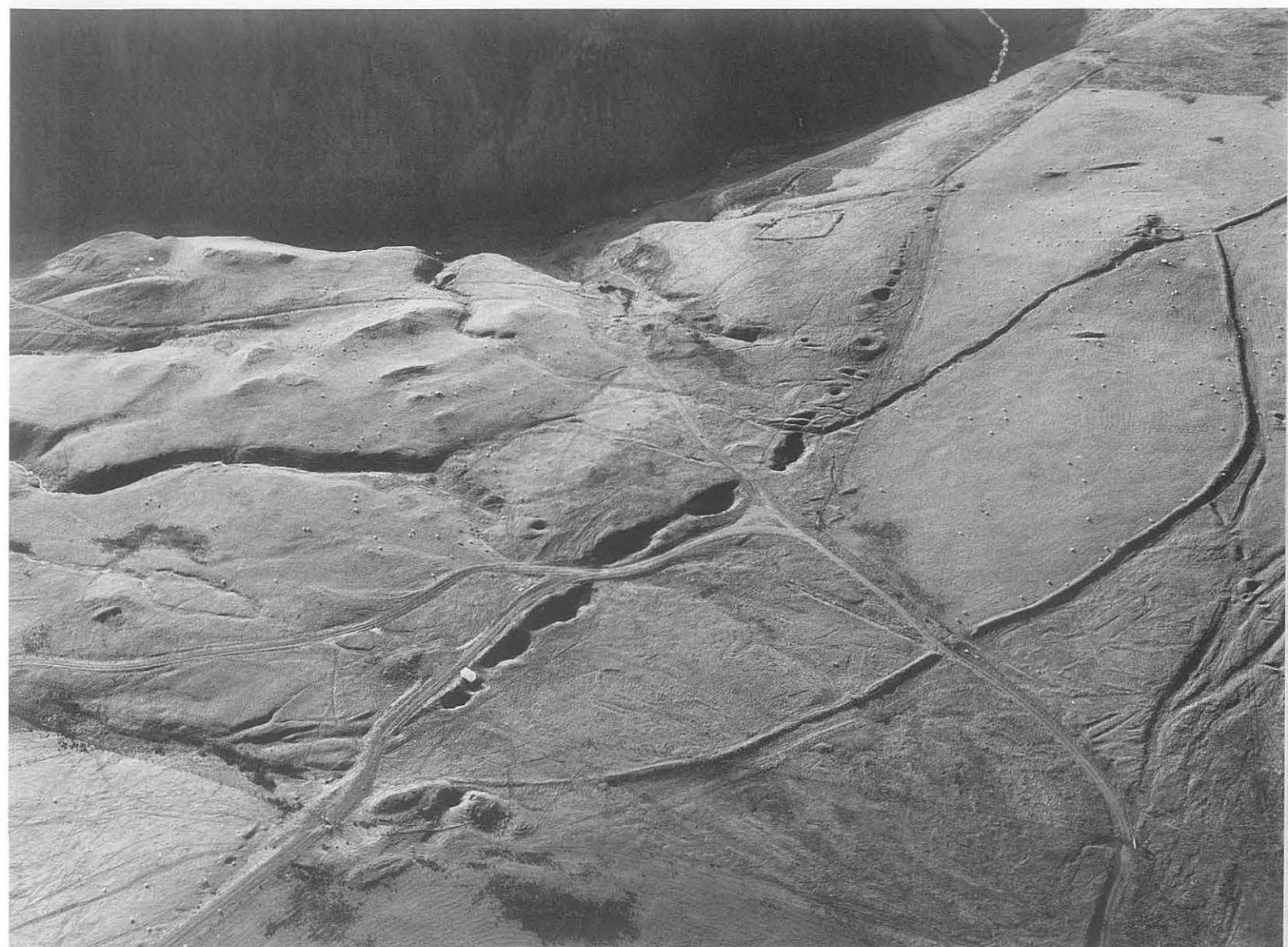
Figure 2 Aerial view of part of the complex mining landscape of the Pen Dylife to the north-west of Llanidloes in mid Wales, described in detail later in the volume. The view shows mine shafts and collapsed workings along the line of a mineral vein, with a hushing channel towards the top right and the site of the engine house towards the lower left. The engine house was the highest to be installed in Wales, a feat requiring fifty horses to haul the equipment to the site ( Crown Copyright: RCAHMW 925090-53 )
