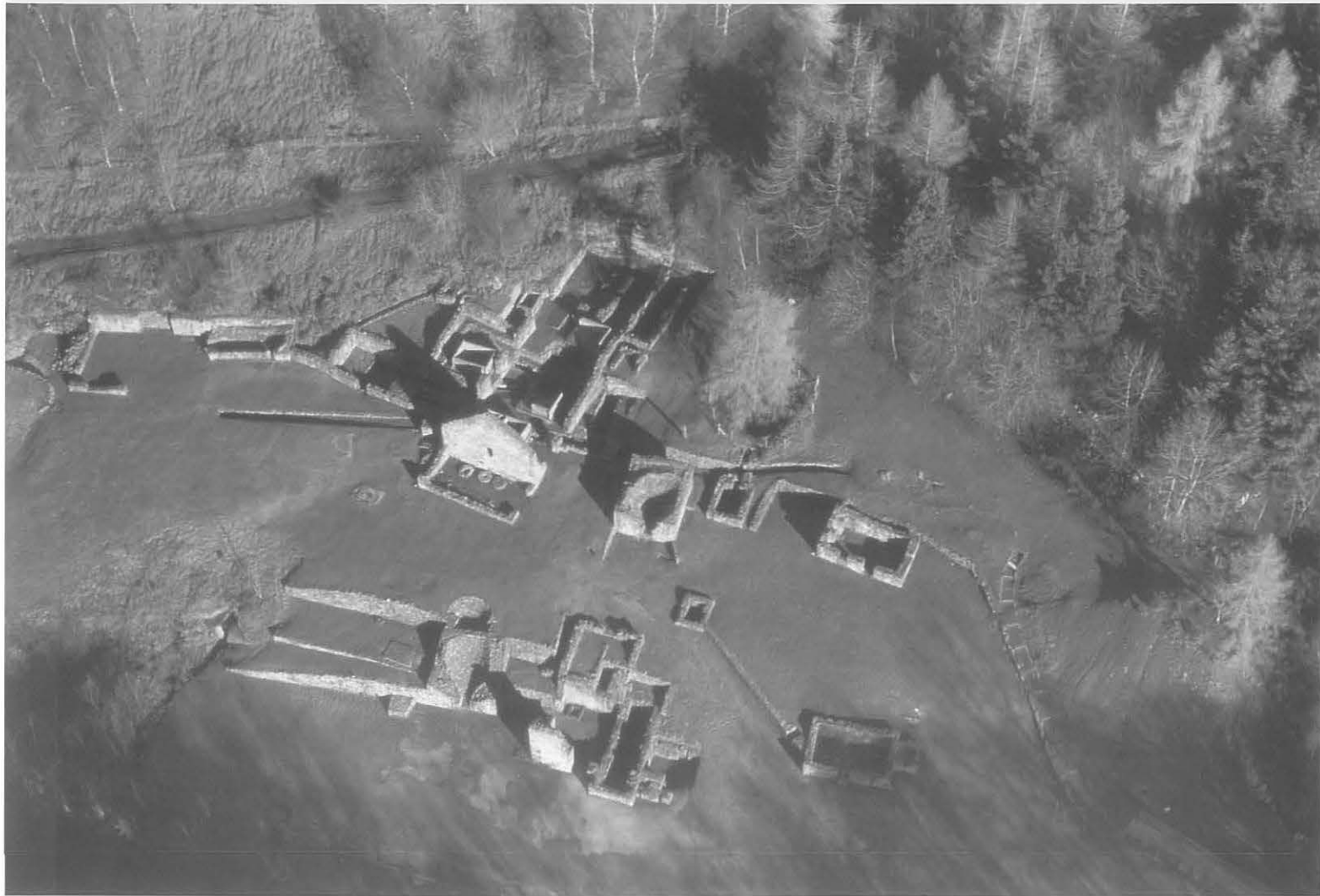
Figure 137 Aerial view of Bryntail mine, Llanidloes, Powys, showing the layout of the 1850s dressing floor below the Western Engine Shaft with the large Barytes Mill erected in about 1870. (Crown Copyright: RCAHMMW 98-CS-903)
