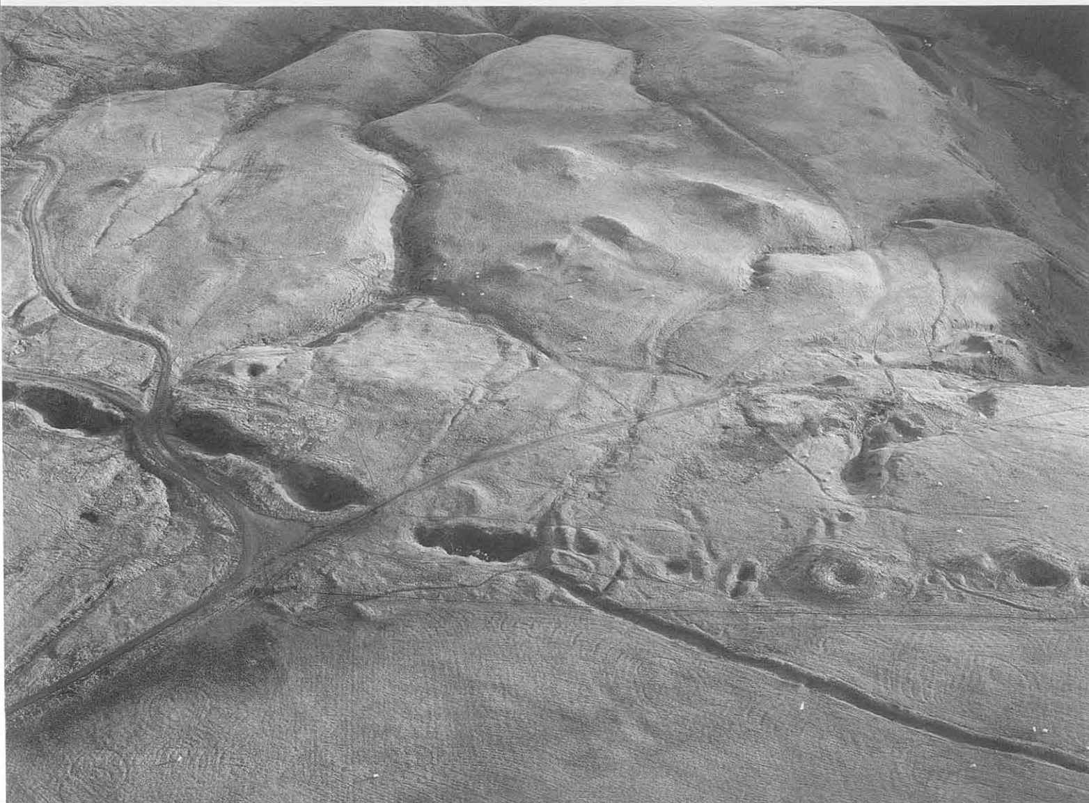
Figure 72 Pen Dylife mine: collapsed workings to the left and hushing channel (18623) and shafts towards the lower right, viewed from the north, with hushing channel bottom right. (Crown Copyright: RCAHWW 945031–44)
