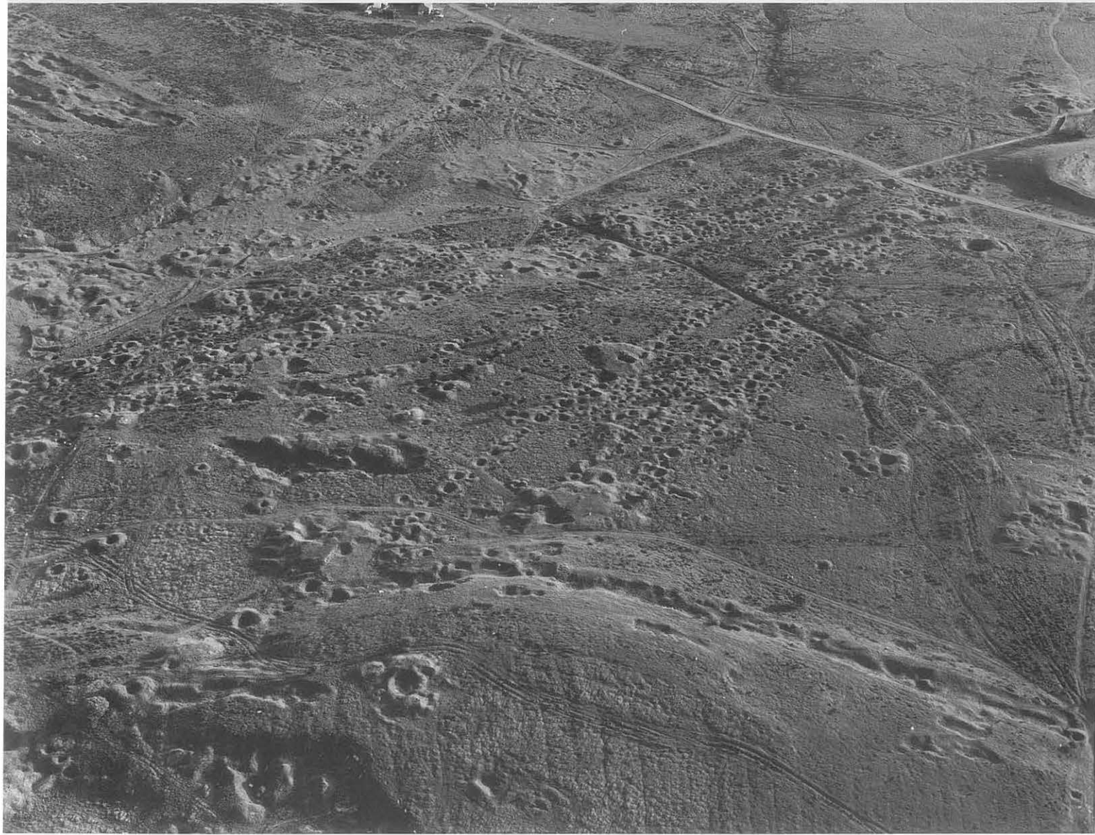
Figure 83 Aerial view of Halkyn Mountain showing the intensive area of mine shafts south-east of Pentre Halkyn (SJ 195715). The area lies to the east of Pant-y-pwll-dwr limestone quarry (see Fig 89), just visible in the top right-hand corner. The lines of shafts, of varying depths, follow rich east-west veins including those known as Billings and Chwarel Las, which were principally worked for lead. The linear workings in the right foreground are probably a north-south cross-cut. Working in this area probably began in the Roman period and continued up to the early 20th century. (Crown Copyright: RCAHMW 935136-45)
