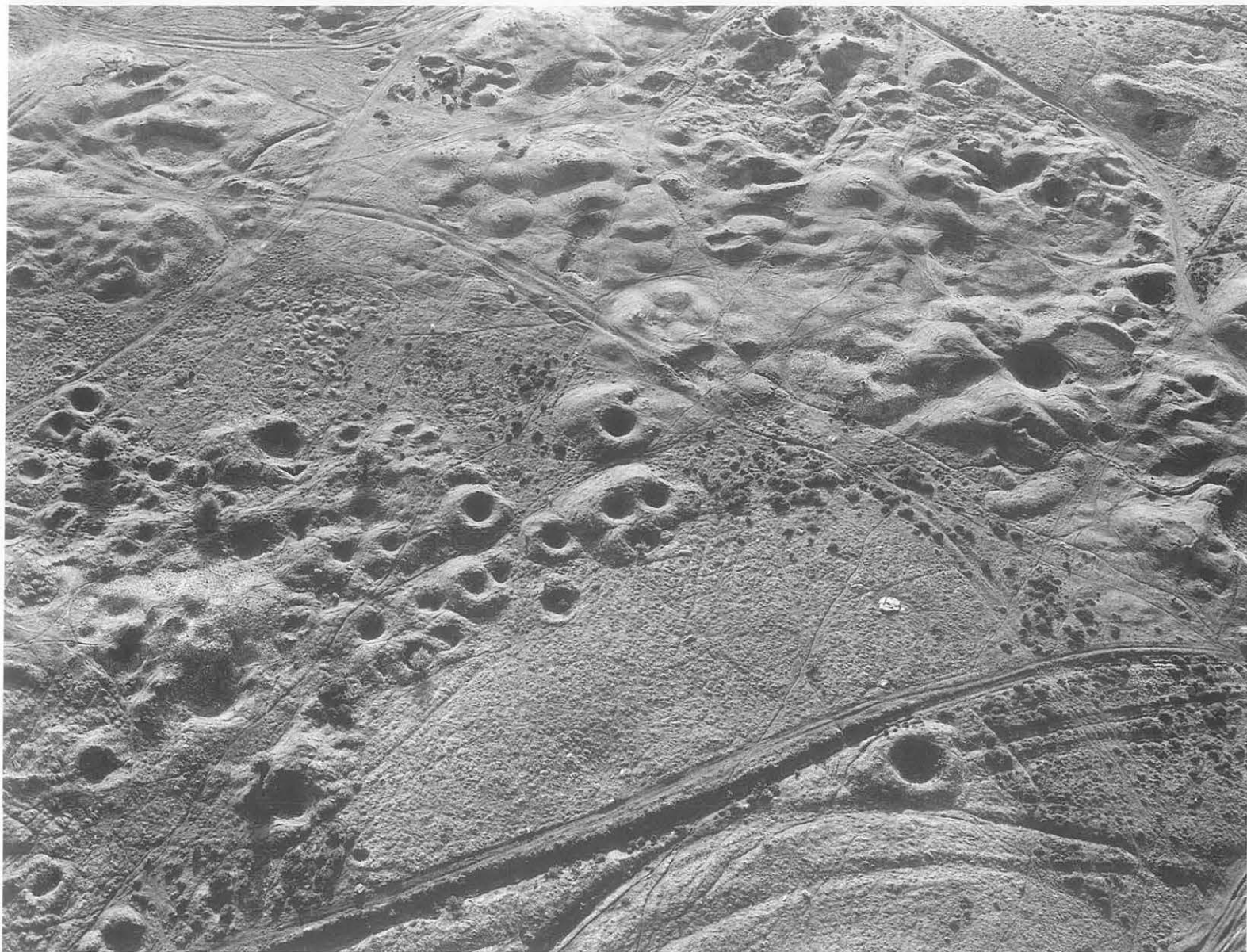
Figure 6 Aerial view of Halkyn Mountain, Holywell, Flintshire. A complex area of shafts, bell-pits and mounds of development waste to the north-east of Rhes-y-cae, probably resulting from mining over a period of six or seven hundred years between the Middle Ages and the early 20th centuries. The ore from the smaller, shallower pits was raised by hand. In the case of the later, larger shafts horse-power or steam-power was generally used. A horse whim circle is visible next to one of the large shafts towards the top right-hand corner of the photograph. An overhead winding drum within a wooden frame, powered by one or two horses, was used here to raise ore from the shaft by means of a pulley set on an A-frame above the head of the shaft. The extensive waste heaps around the shaft suggest that ore may also have been processed in this area. ( Crown Copyright: RCAHWW 935136-48 )
