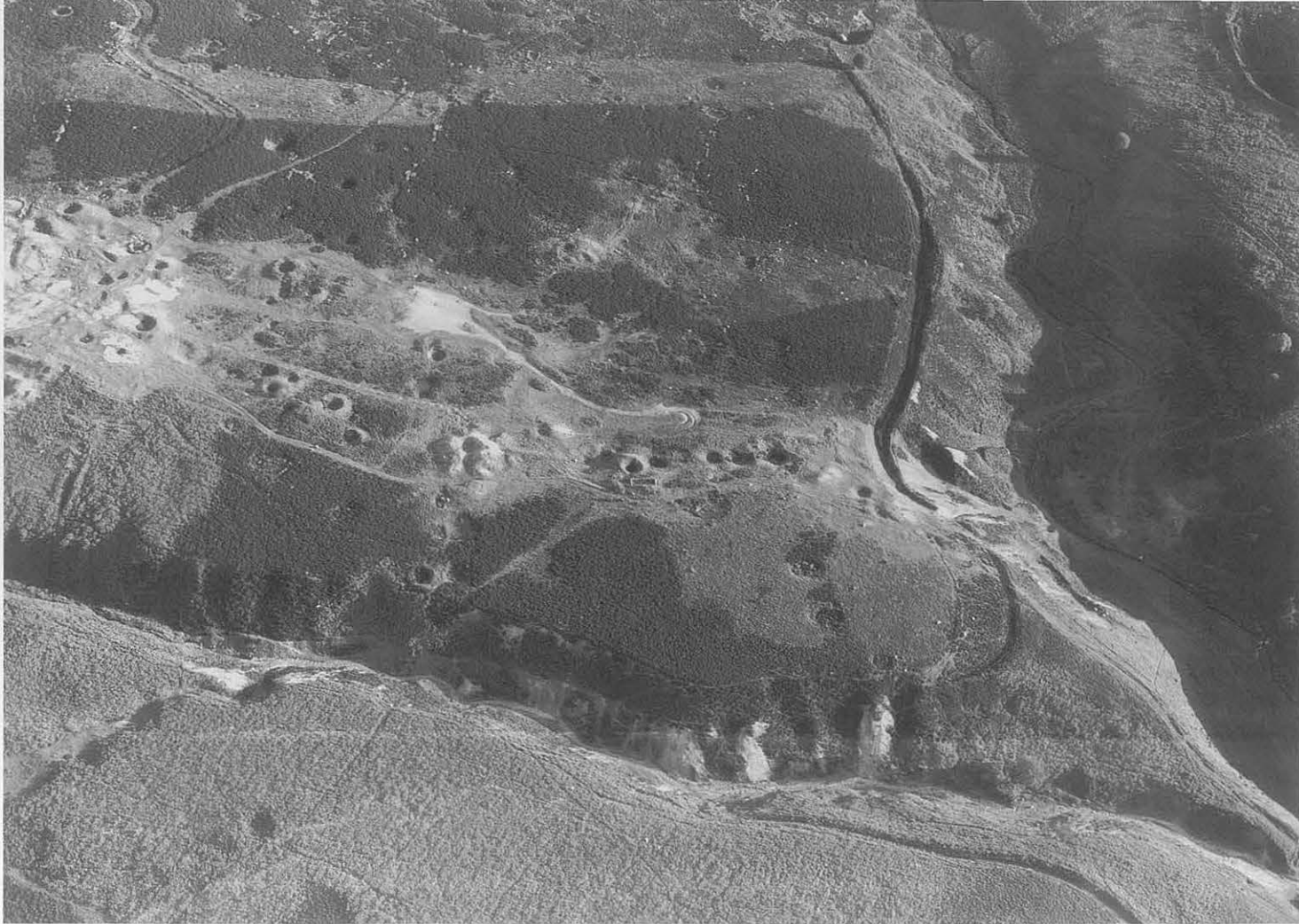
Figure 123 Aerial view of Pool Park mine, seen from the north-east. The mine shafts are strung out along the side of the stream in the foreground which feeds the Aber Sychnant stream, visible to the right. In the moorland beyond the mine is a scatter of natural sink-holes which join an underlying cave system in the limestone connected to the underground mine workings. The substantial leat running along the left-hand edge of the Aber Sychnant Valley is of late 19th-century date. It was formerly carried on a timber aqueduct over the stream in the foreground and fed two reservoirs (SJ263515) above the Minera mines, where the water was used to drive machinery on the dressing floor and to supply the engine house boilers. ( Crown Copyright: RCAHMW 935151-57 )
