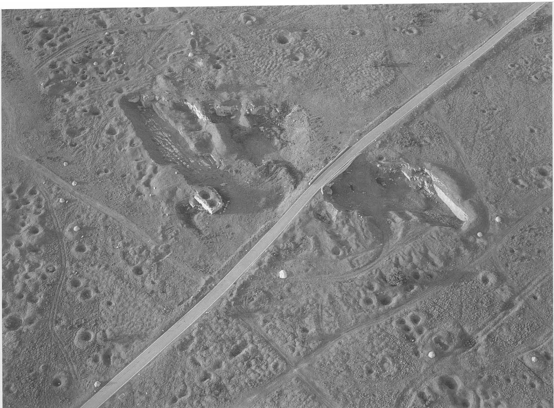
Figure 81 Aerial view of lead mining and limestone quarrying to the north of the road between Rhys-y-cae and Halkyn. Many of the shafts in this area have little development waste and were therefore probably either fairly shallow or have been backfilled. Some have concrete beehive cappings. The quarries are associated with the pair of limekilns at the centre of the photograph. (Crown Copyright: RCAHMMW 935136-51)
