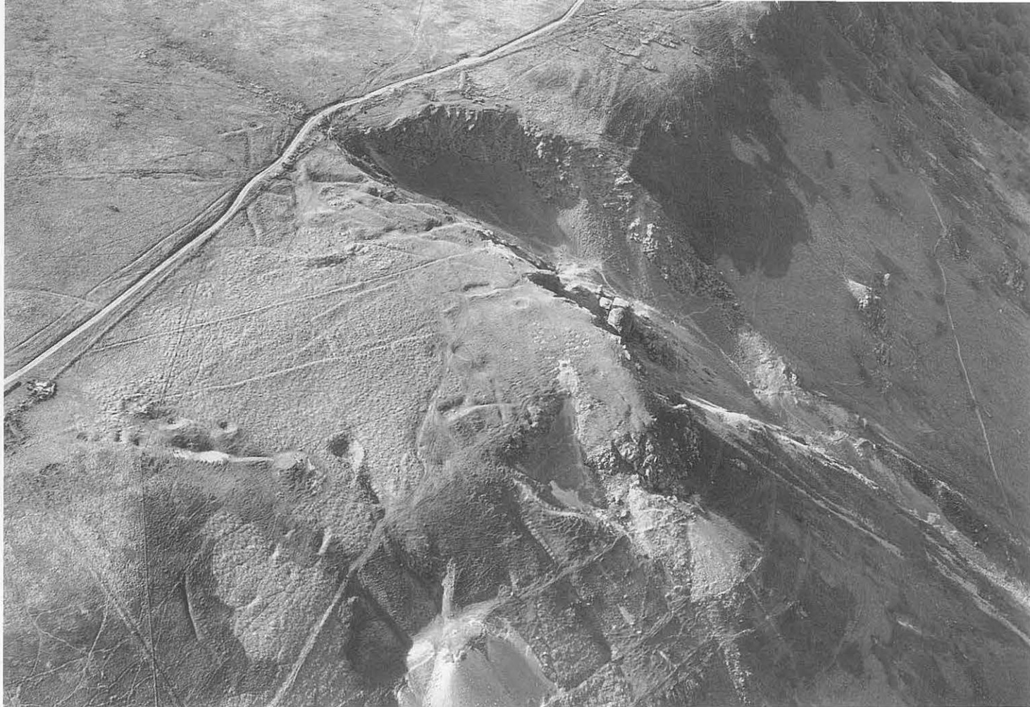
Figure 7 Aerial view of Craig-y-Mwyn mine, Llanrhaeadr-ym-Mochnant, Powys, showing the open-cast with associated hushing channels, leats and reservoirs. (Crown Copyright: RCAHMMW 935097-52)
