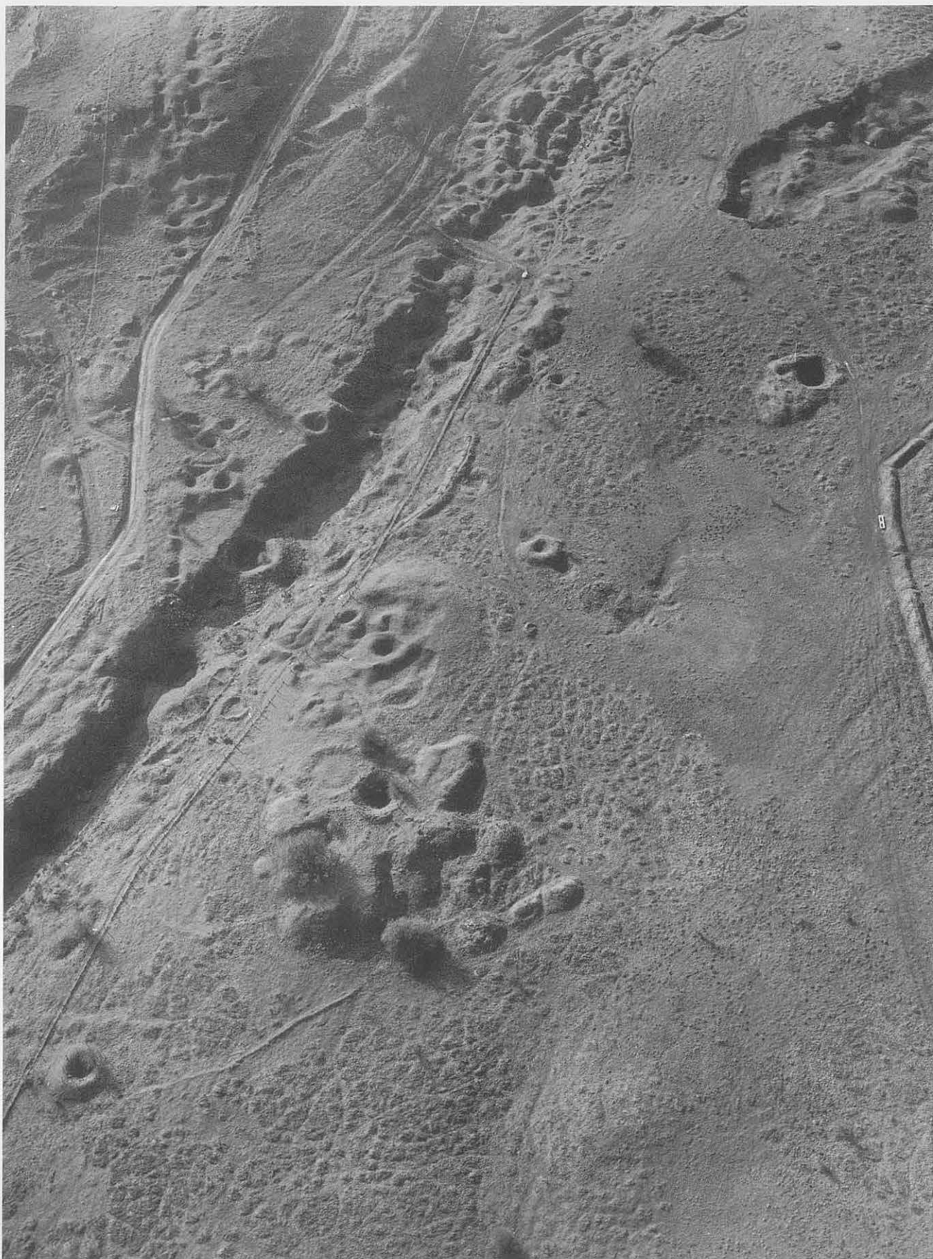
Figure 104 Aerial view showing a shaft and whim circle (18946, 18810, see Fig 106) on the north side of the Hush, visible towards the centre foreground. The area in which the shaft lies is shown on Brenton Symonds's map of 1865 as falling within the Ragman mine sett, and probably represents mid to late 19th-century workings. The boundary with the West Minera mine, which included the Hush, lay just beyond. (CPAT 90-MB-290)
