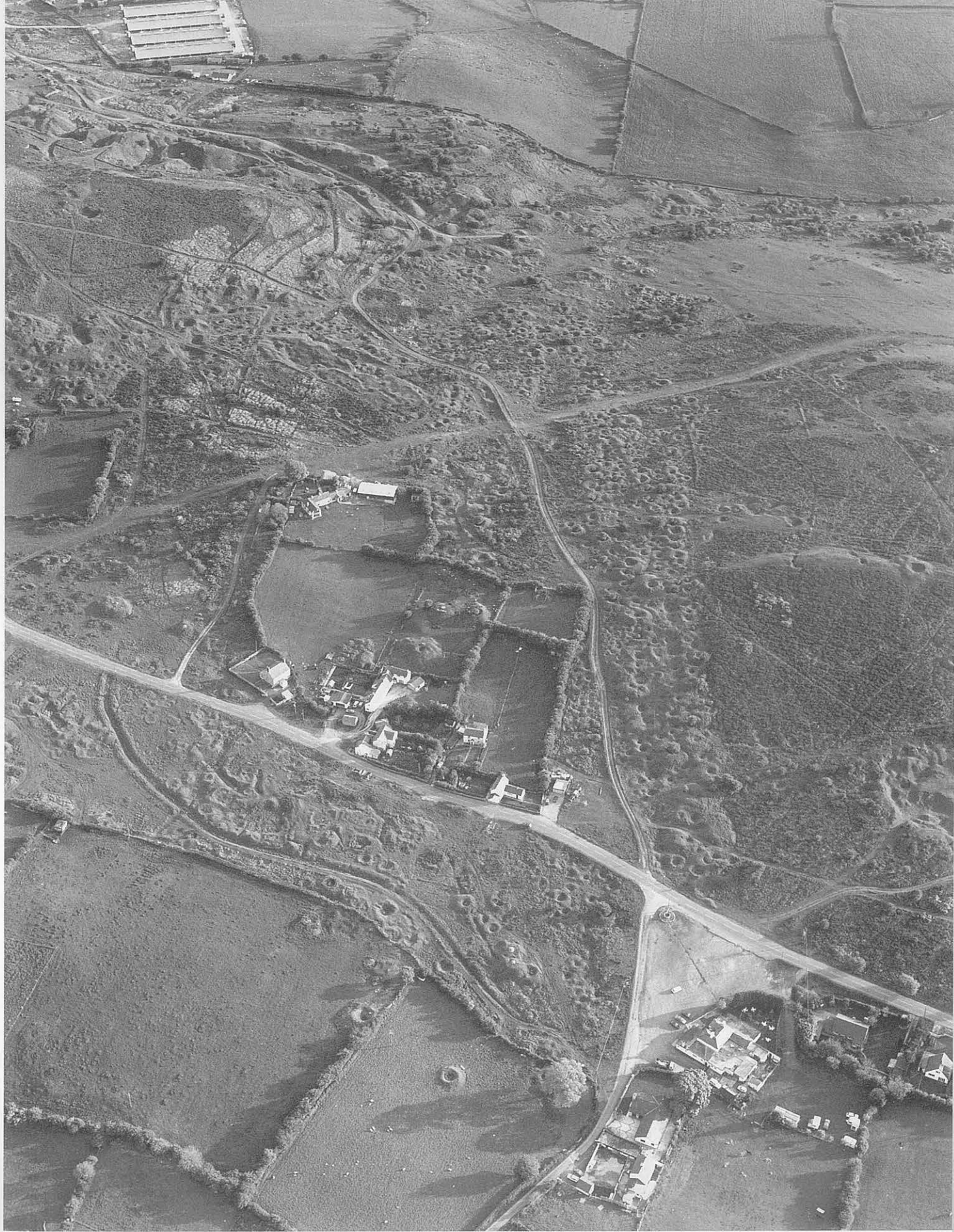
Figure 87 Aerial view of Halkyn Mountain showing lines of shafts running along the rich Pwll-clai and Pant-y-pydw veins, Holywell Common. The settlement of Pwll-clai (SJ186738), seen from the north-east, lies at the centre, on the far side of the road between Brynford and Pentre Halkyn (see Fig 88). Fewer workings are visible in the fields to the lower right-hand corner, suggesting that this area has been reclaimed. A curving ditch just below the road was formerly a leat which served water-powered machinery at the Pwll-clai dressing floors. (Crown Copyright: RCAHMW 935135-56)
