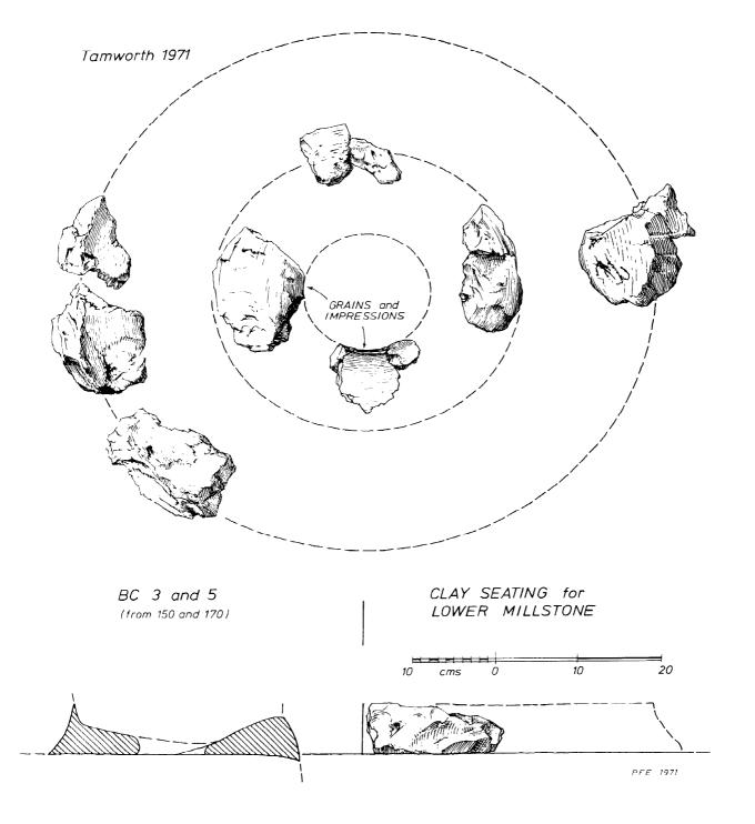
Figure 63 Clay seating for lower millstone, BC3 and 5
