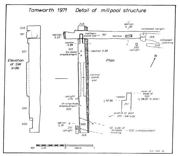
Figure 89 Detail of millpool structure; NW and SW walls and other features
