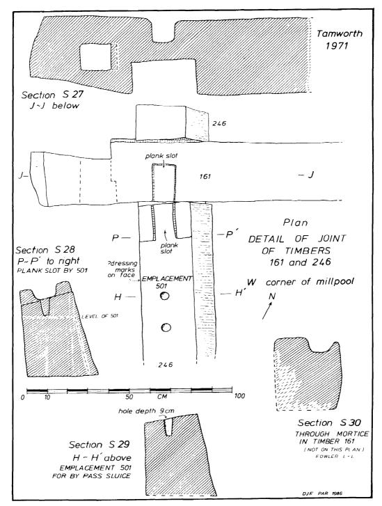
Figure 90 W corner of millpool: detail of joint of timbers 161 and 246, with sections S27-S30 of both
