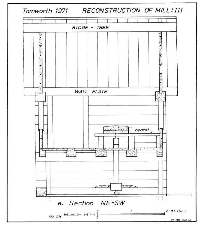
Figure 97 Reconstruction of mill III: e) section NE-SW (F W B Charles)
