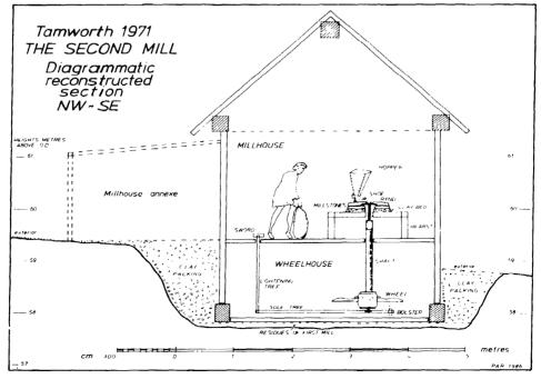
Figure 94 The second mill: diagrammatic reconstructed section NW-SE
