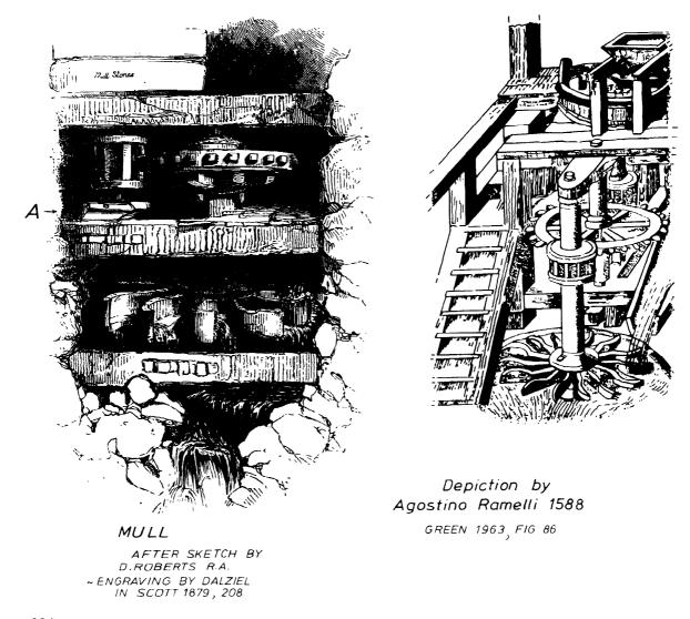
Figure 104 Geared horizontal-wheeled mills, on Mull (in Scott 1879); by Ramelli 1588
