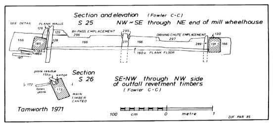
Figure 88 NW-SE through NE end of mill wheelhouse, section and elevation S25; and SE-NW through NW side of outfall revetment timbers, section S26
