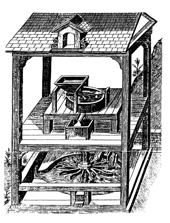
Figure 105 Drawing of a horizontal-wheeled mill (by Ramelli 1588)
