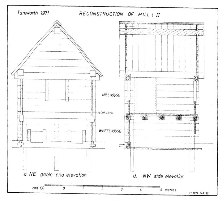
Figure 96 Reconstruction of mill II: elevations of c) gable end and d) NW side (F W B Charles)
