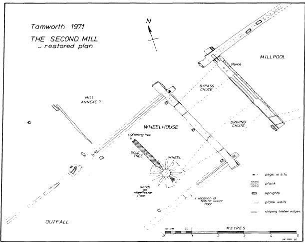
Figure 80 The second mill: restored plan of wheelhouse and millpool
