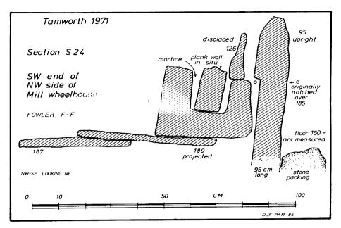
Figure 87 SW end of NW side of mill structure, section of timber, S24
