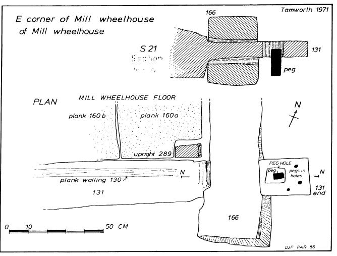
Figure 84 E corner of mill wheelhouse; detail of joint of timbers 166 and 131, in plan and section S21
