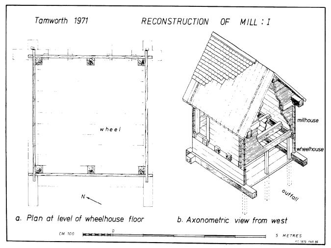
Figure 95 Reconstruction of mill I: a) plan at level of wheelhouse floor; b) axonometric view of mill from W (F W B Charles)
