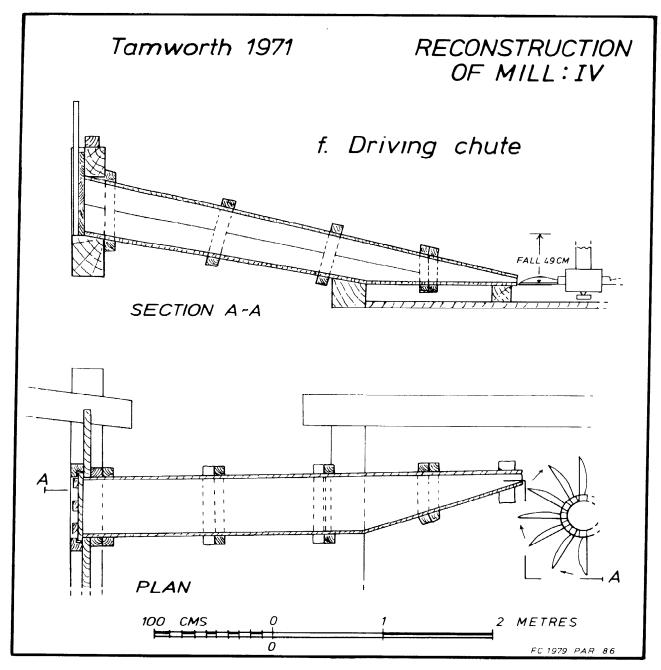
Figure 98 Reconstruction of mill IV : f) driving chute (F W B Charles)
