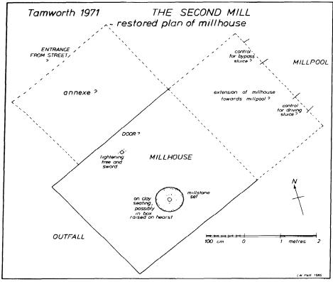
*Figure 81 The second mill: restored plan of millhouse*
