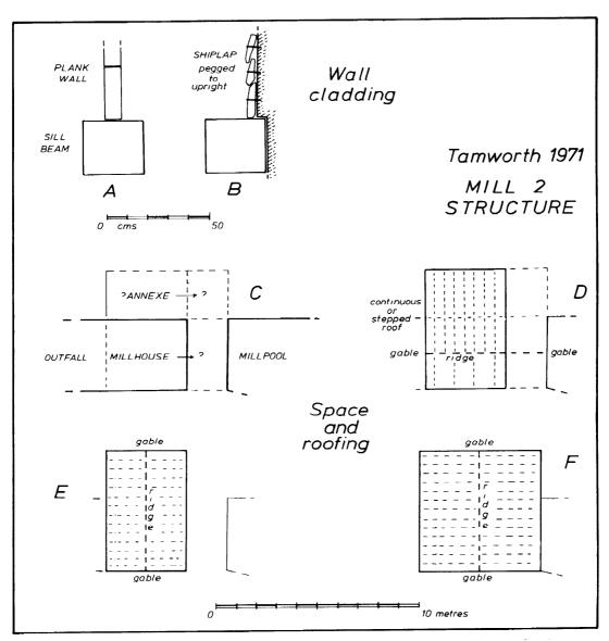
Figure 92 Mill 2 structure: wall cladding (A, B), space and roofing (C-F)
