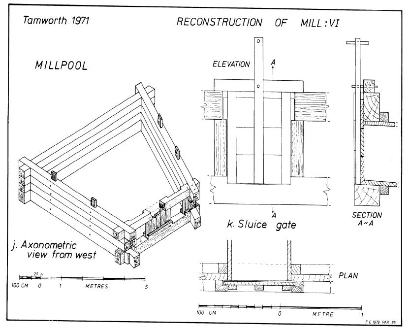
Figure 100 Reconstruction of mill VI: j) millpool, axonemetric view from W; k) sluice gate
