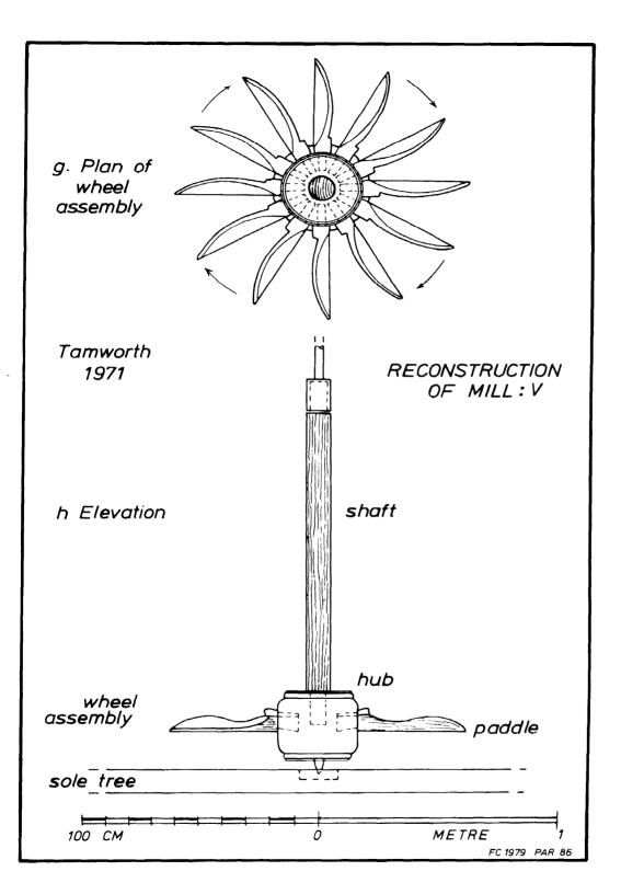
Figure 99 Reconstruction of mill V: g) wheel-assembly; h) elevation (F W B Charles)
