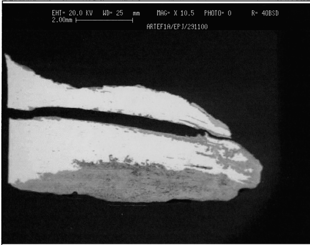
ARTE1A: SEM-BS image of sample showing (at least) two strips of metal originally welded but presently separated by corrosion (gap). Dark grey area is a layer of surface corrosion (bar = 2 mm)
