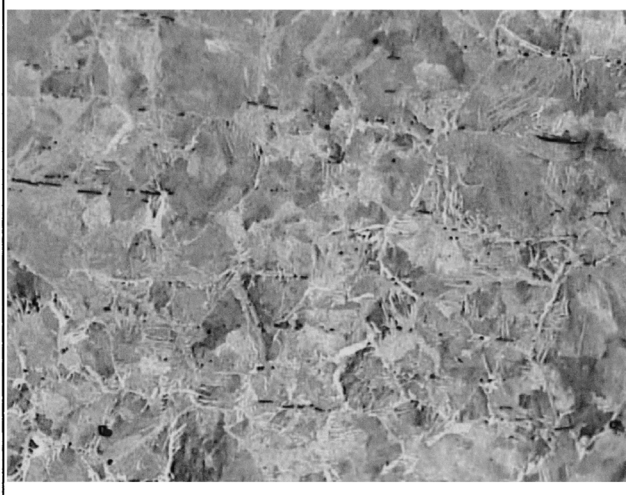
Illus 38 Microscopic images (SEM-BS) of samples from the edge (ARTE1A) of the shaft-hole axe
