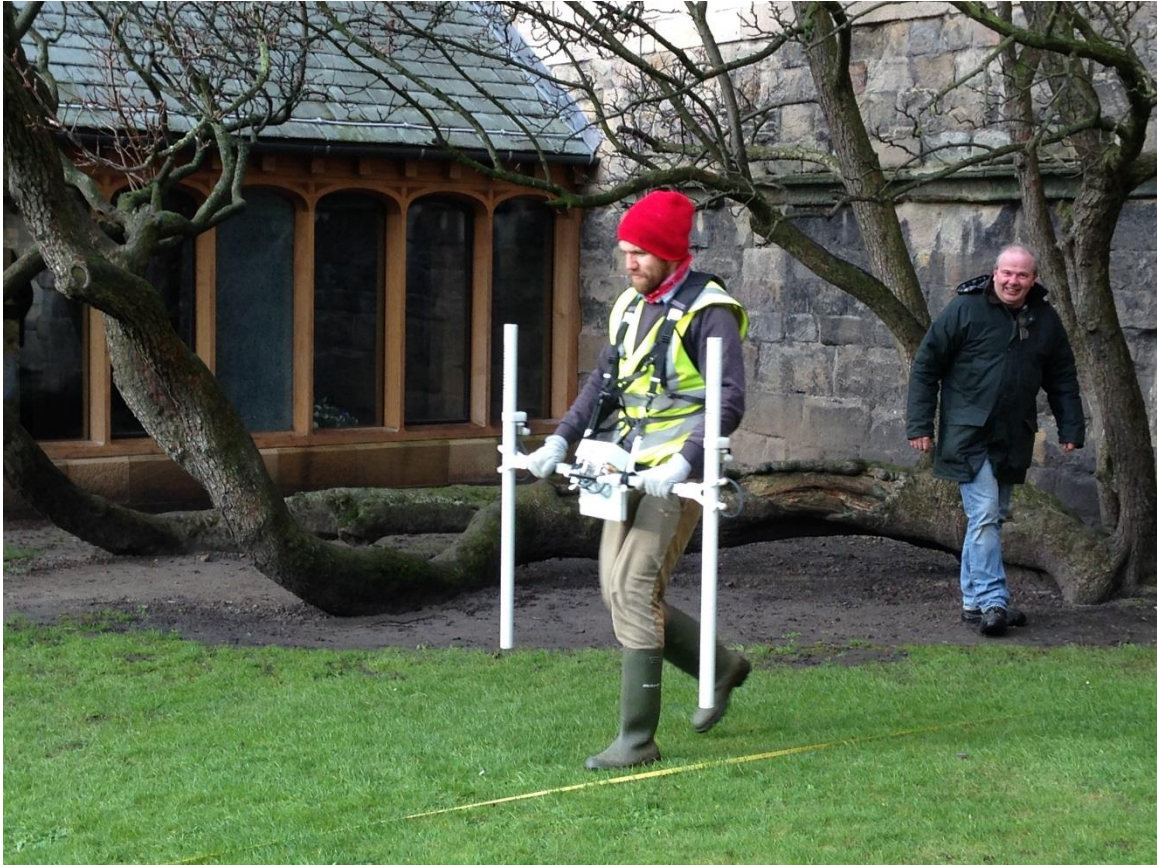
Figure 19: D. Astbury taking gradiometer readings in area 1a (Cloister) 9/02/2016 (Photo: S. Hueglin)
