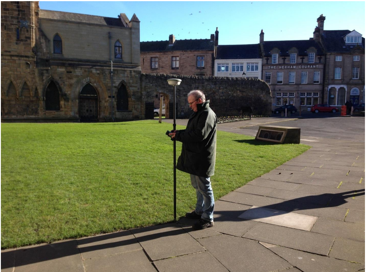
Figure 11: All areas were located by differential GPS. A. Turner on 11/02/2016 in area 1a (Cloister) (Photo: S. Hueglin)
