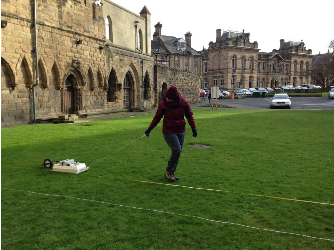
Figure 16: S. Hueglin pulling the GPR sled across area 1a (Cloister) 9/02/2016 (Photo: D. Astbury)
