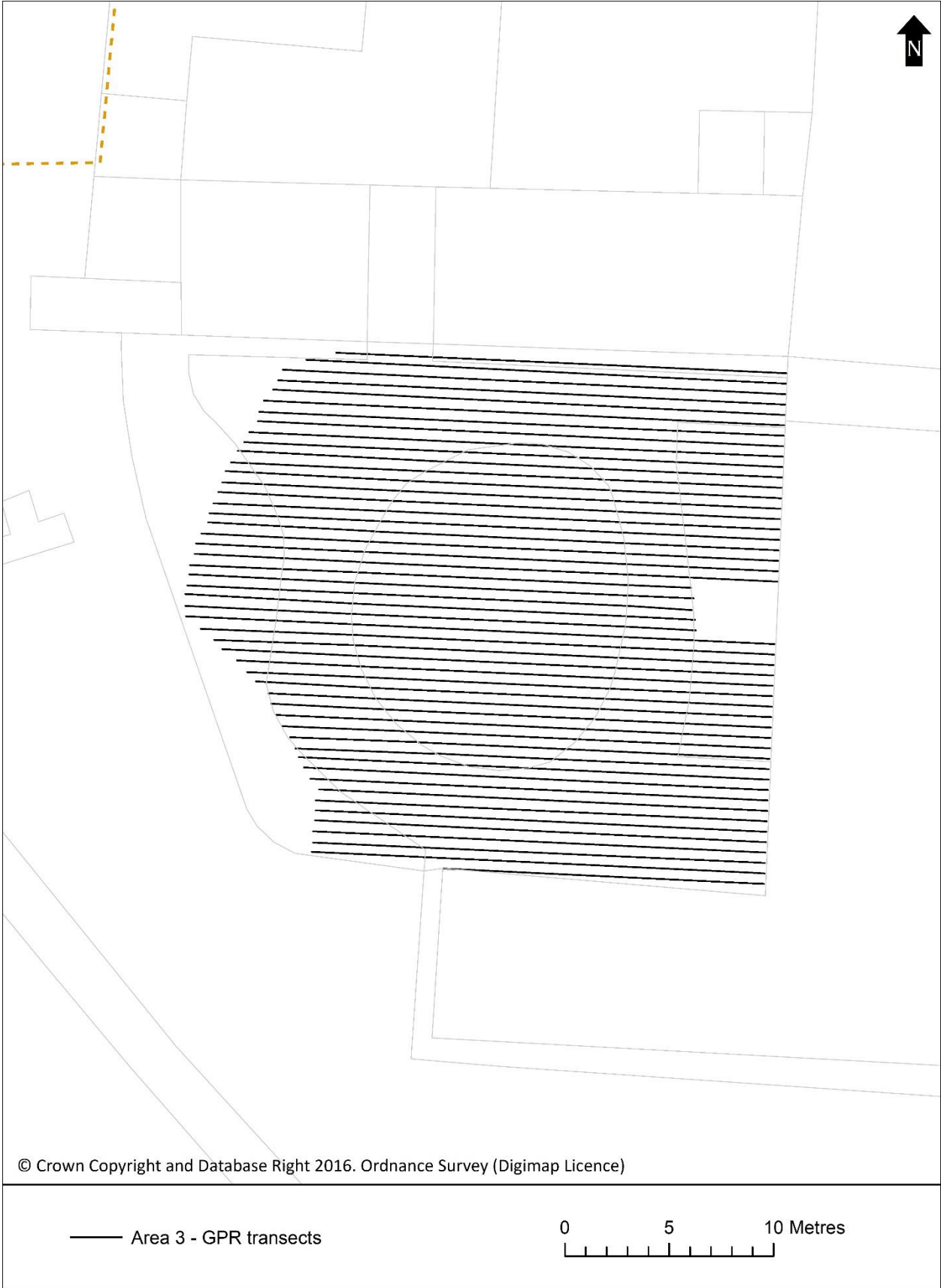
Figure 14: Ground Penetrating Radar, survey transects in area 3 (Prior's Court) (Graphics: A. Turner).
