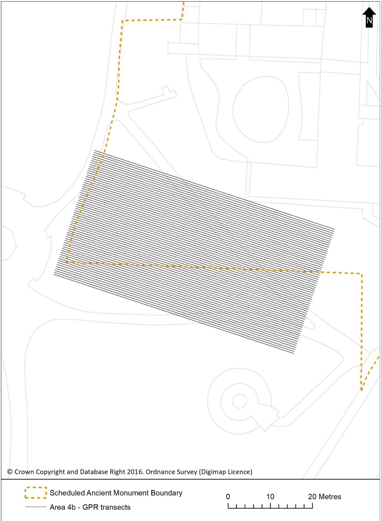
Figure 15: Ground Penetrating Radar, survey transects in area 4b (Park) (Graphics: A. Turner).
